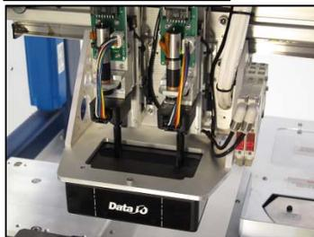
**Dual-alignment-on-the-fly is done with a head-mounted laser-align system originally designed for SMT placement machines**
