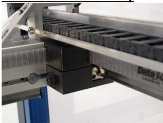
**The servo-driven H-bot gantry, coupled with dual-loop encoders and kinematic algorithm achieves the highest accuracy and throughput**
