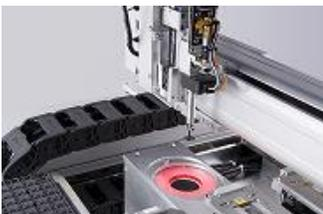
**Camera vision:** alignment as seen in figure 1 is the safest and most efficient way to ensure precise component placement into sockets and I/O media while protecting the lead integrity of each device.
