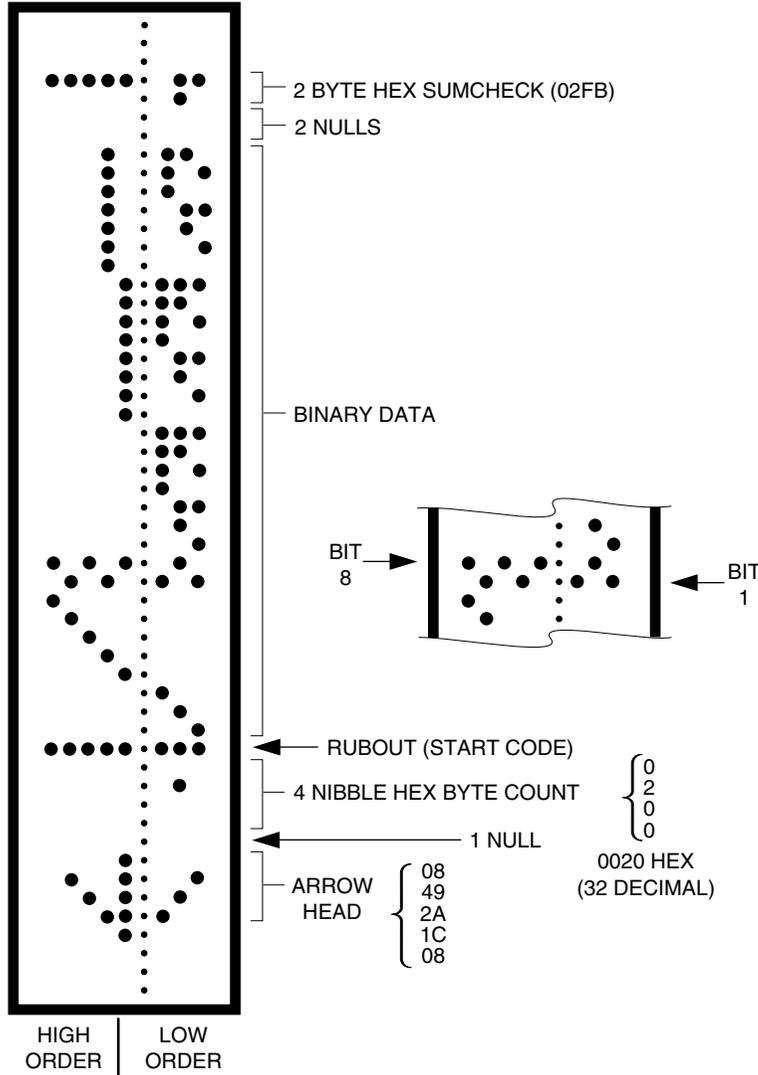
The programmer stores incoming binary data upon receipt of the start character. Data are stored in RAM starting at the first RAM address specified by the Memory Begin Address parameter and ending at the last incoming data byte.
