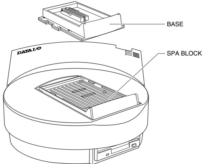
2. Mildly dampen a small section of a lint-free cloth with a DeoxIT pen (Data I/O P/N 570-5500-901) and gently rub the dampened cloth across all the pins on the SPA block.
