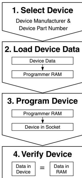
Select the manufacturer and part number of the device you will be using so the programmer can perform device operations with the appropriate programming algorithm.
