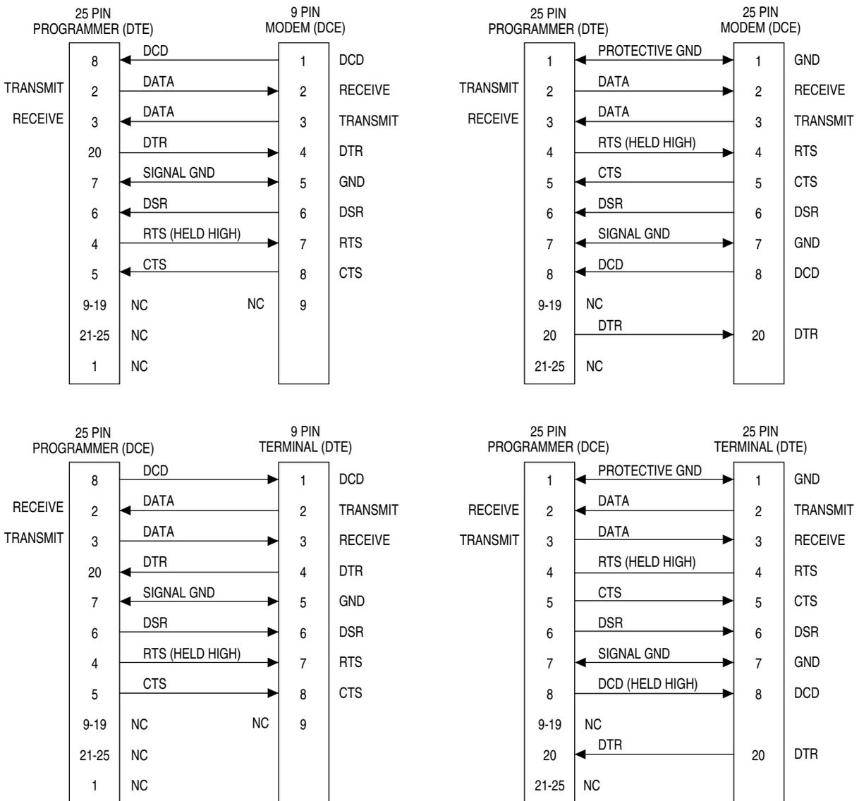
The minimum hookup includes Pins 2, 3, and 7. Pins 1 and 7 are tied together.
