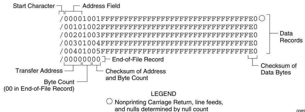
Data are output from the programmer starting at the first RAM address and continuing until the number of bytes in the specified block has been transmitted. The programmer divides output data into records prefaced by a start character and an address field for the first byte in the record.
