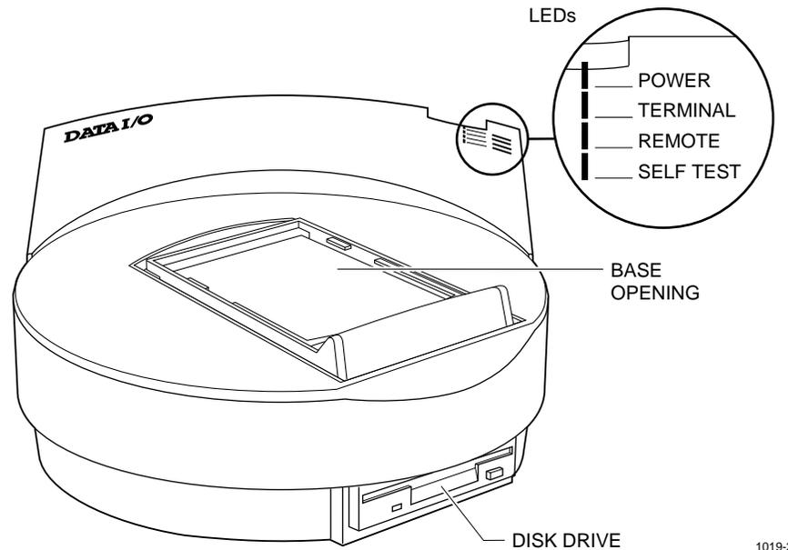
**Power LED**—When this lamp is lit, the power is on.
