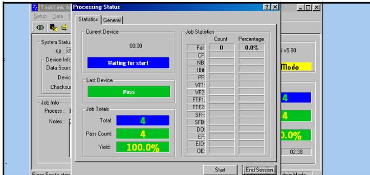
15. During the processing, the number of successfully programmed devices and total number of attempts is displayed. The **Last Device** box displays "Pass" on a green background or a message that describes failure on a red background.
