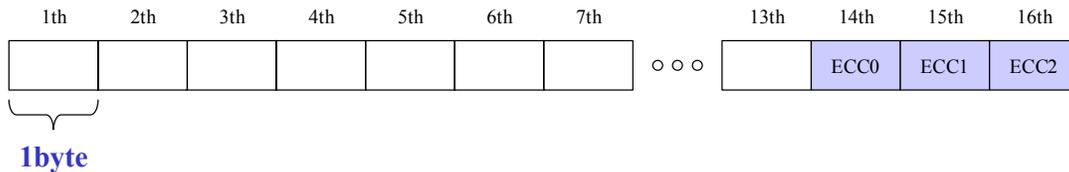
Note that if “ECC” is selected from the “Spare area” drop down list, the rest of the spare area is left blank (FFh); the spare area cannot be used for both ECC and data storage. For details on the method used to calculate the ECC value, see the code example on Samsung’s web site at <http://www.samsungusa.com/download/semiconductors/flash/eccalgo.pdf>.
