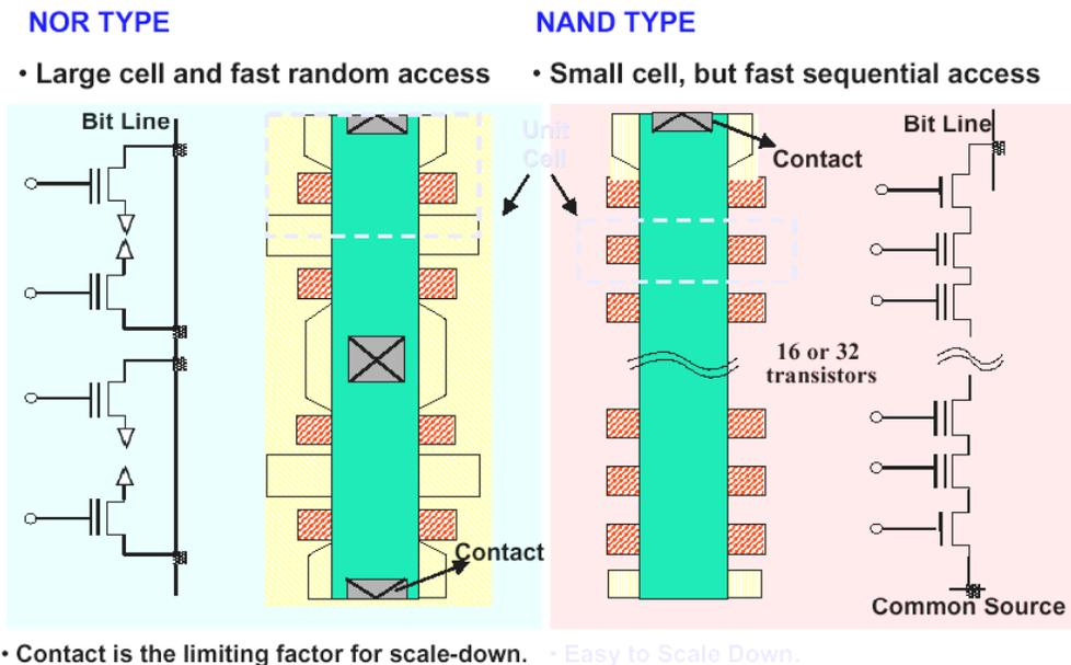
Figure 1: NAND and NOR cell comparison (from Samsung application note).
