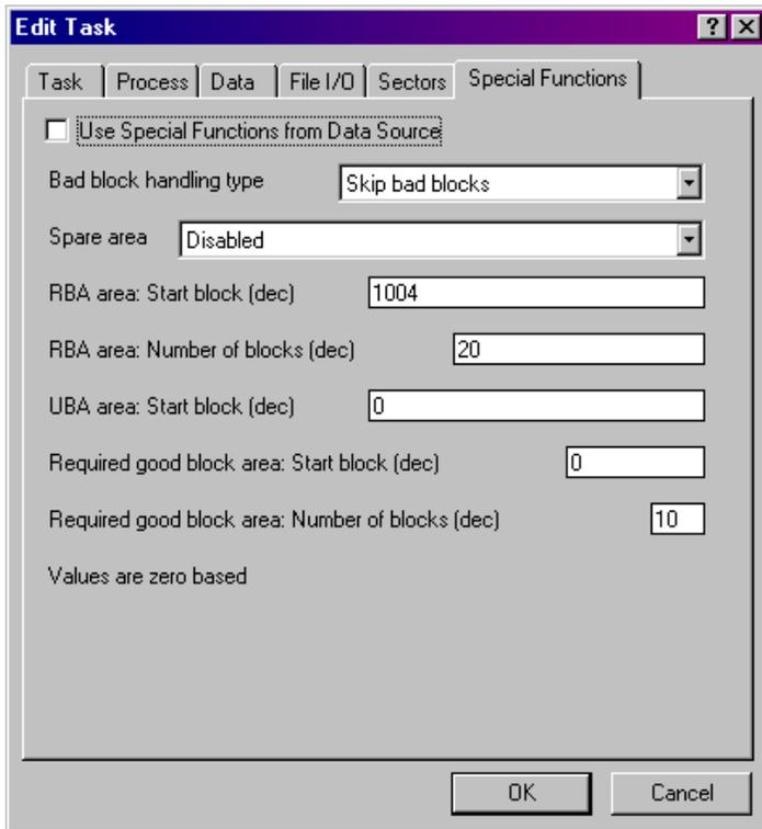
Figure 4: Special Functions for NAND devices.
