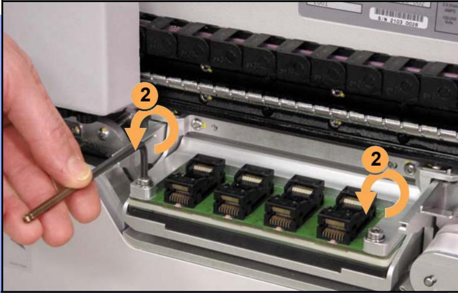
To change the Socket Adapter (with the Actuator Plate removed):
