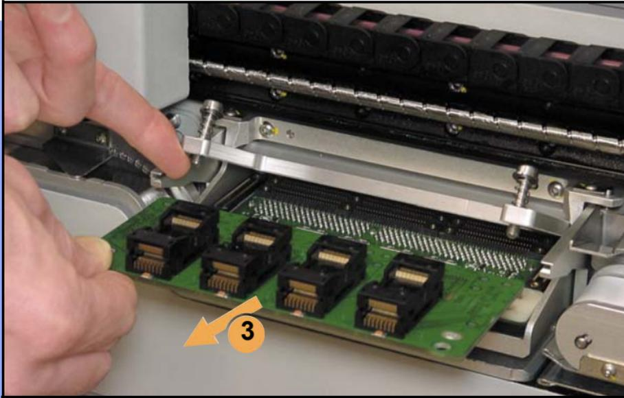
3. Without touching the gold contact surfaces on the bottom of the adapter, lift the adapter free.
