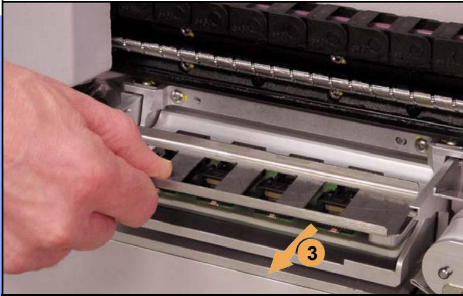
3. Pull the Actuator Plate to slide it out of the grooved brackets.
