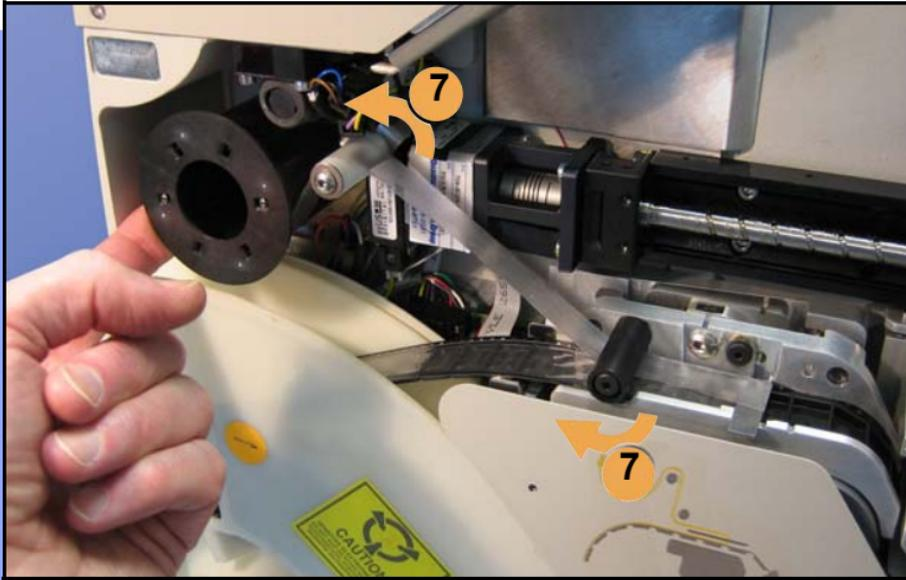
6. When the tape is advanced just past the Peel Bar, separate the cover tape from the device tape.
