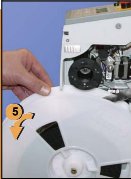
If the tape jams, an error message displays and the blue lamp illuminates. To clear the tape path:
