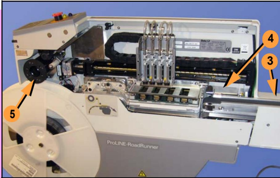
3. Clear away excess devices from the conveyor belt.
