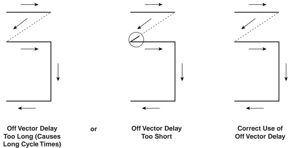
Figure 2-15 Off Vector Delay settings
