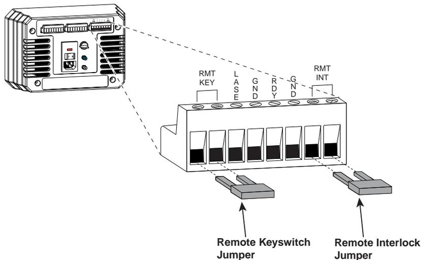
Figure 1-5 Auxiliary Signal terminals
