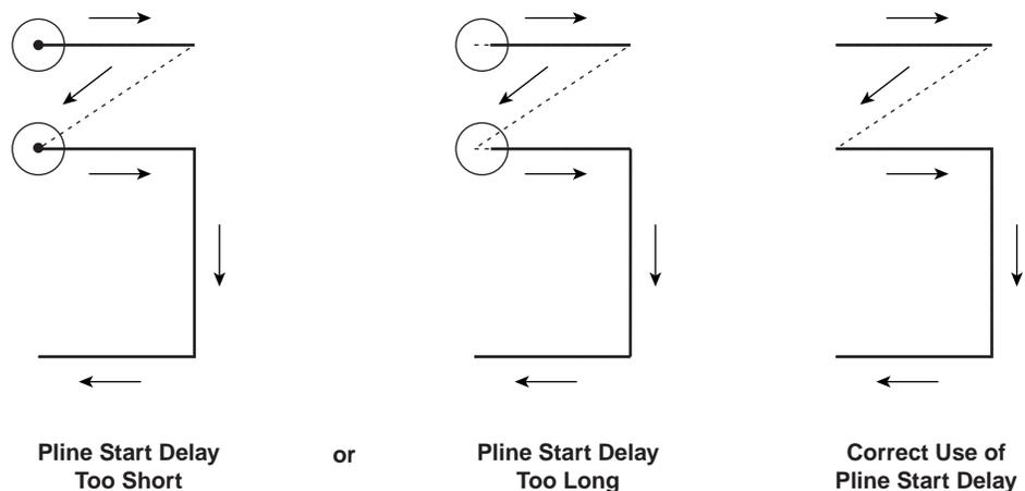
Figure 2-12 Pline Start Delay settings
