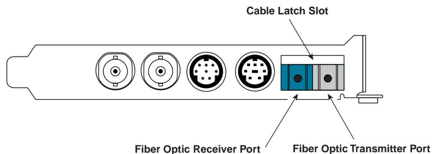
Figure 1-4 Fiber Link Card connectors
