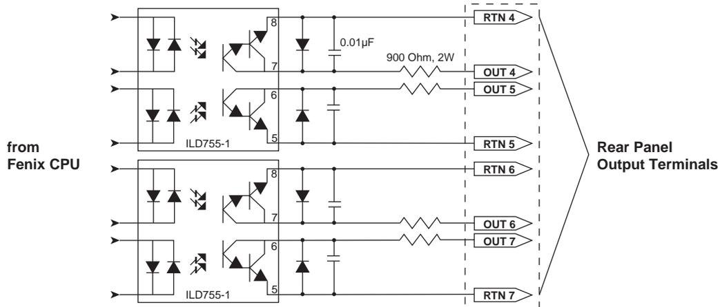
Figure 3-3 Output circuit
