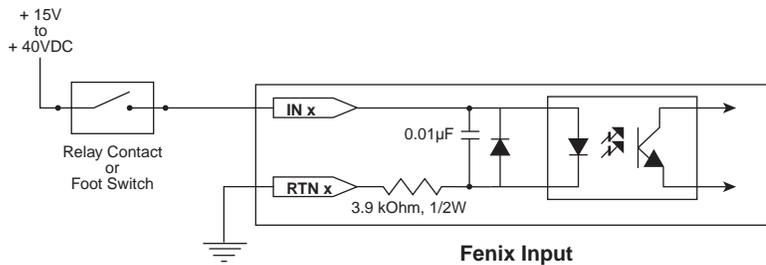
Figure 3-7 Relay or foot switch input
