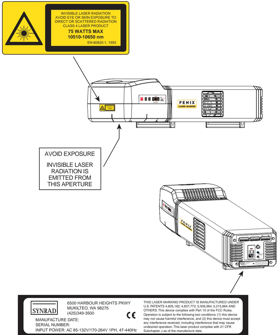
Figure i Fenix hazard label and CE label locations
