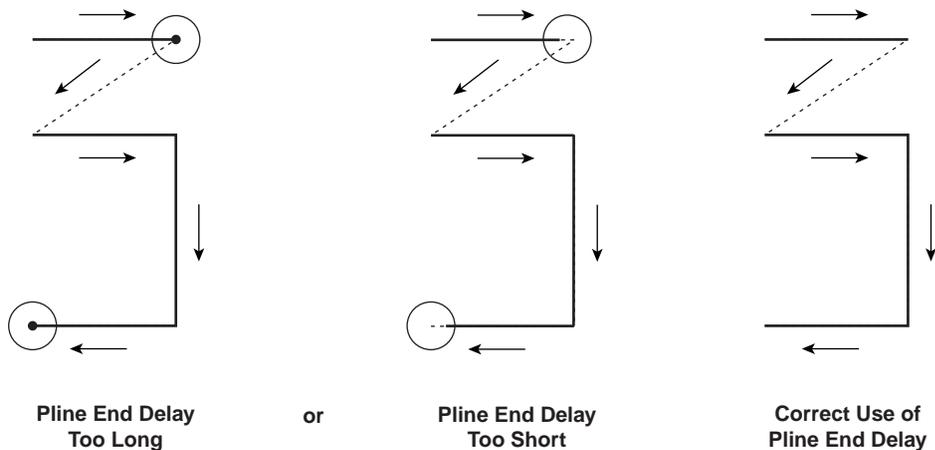
Figure 2-13 Pline End Delay settings
