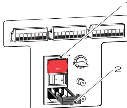
Figure 4-2 AC line fuse location
