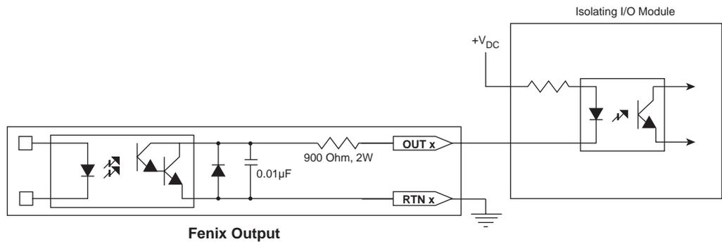
Figure 3-8 Output to isolated I/O module
