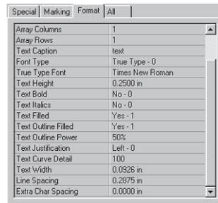
Figure 2-18 Format tab text properties
