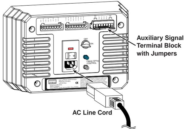
Figure 1 Fenix quick start connections
