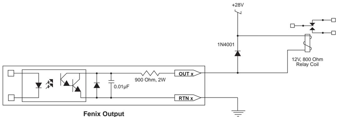
Figure 3-9 Output to relay driver
