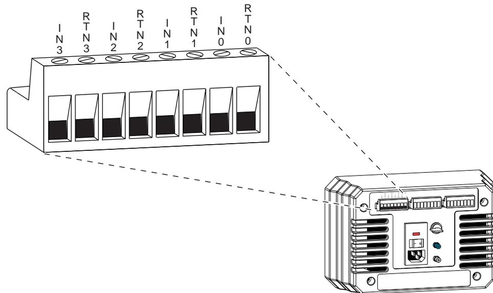
Figure 3-2 Input terminal pinouts
