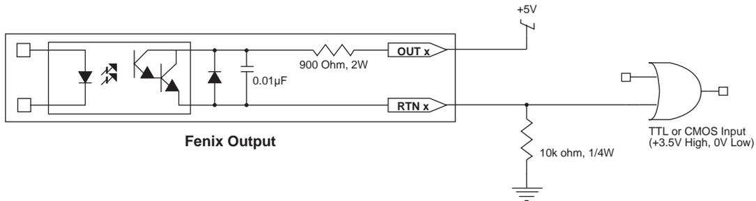
Figure 3-10 Output to TTL or CMOS logic interface
