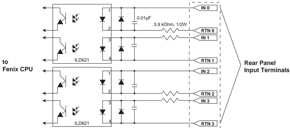
Figure 3-1 Input circuit
