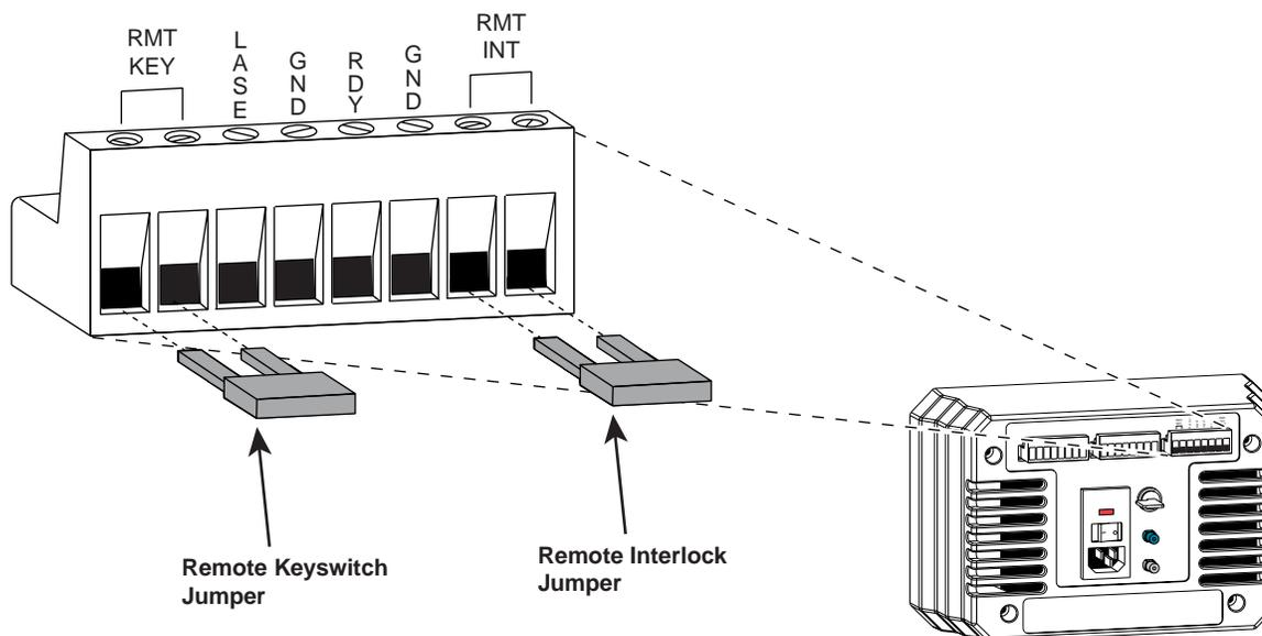
Figure 3-5 Auxiliary Signal connector
