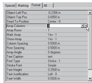
Figure 1-15 Setting number of Array Columns
