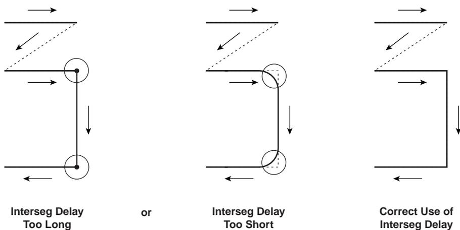
Figure 2-14 Interseg Delay settings
