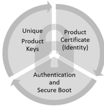
Figure 2 – Components of a Root of Trust
