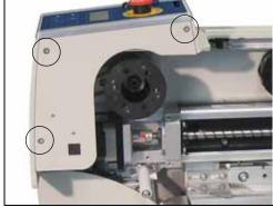
Figure SX-26—Corner Panel Cover with screw locations circled.
