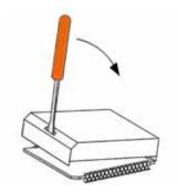
Figure SX-47—Removing the cap from the base.
