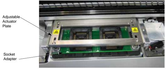
Figure SX-55—Actuator Plate Assembly and Socket Adapter
