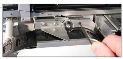
Figure SX-6—Adjusting the 32/44 mm Tape-In Module: loosening the Centering Bar screw. The Position Locking screw (circled) is already loosened.
