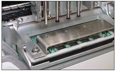
Figure SX-41—The Programmer Module Alignment Tool Installed on the Programmer in place of a Socket Adapter. (PROBE TIPS MUST BE REMOVED PRIOR TO ALIGNMENT PROCEDURE.)
