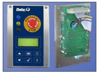
Figure SX-25—Control Panel Module, front and back
