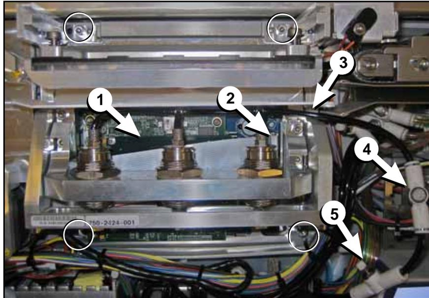
Figure 4-41—Programmer Module with mounting screws circled (with the lower left one hidden by cables).
