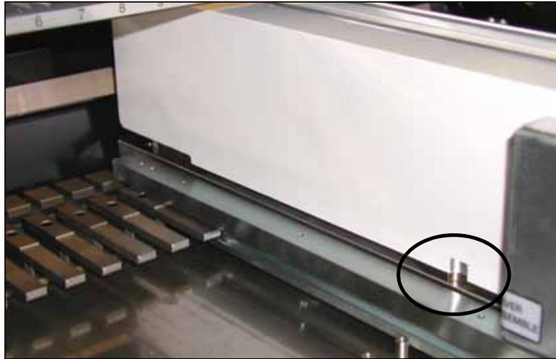
*Figure 2-10—The dowel on the Adapter (circled) mates with RoadRunner3.*
