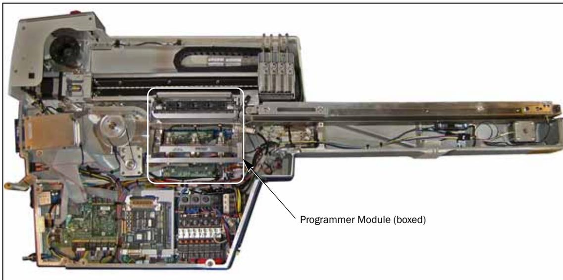
Figure 4-57—Parts in the Programmer Spares Kit; RoadRunner3
