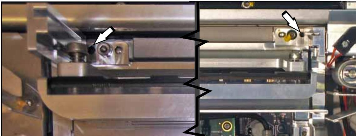
Figure 4-45—Programmer Module Alignment Screw. The Left Screw (left) is shown closer.
