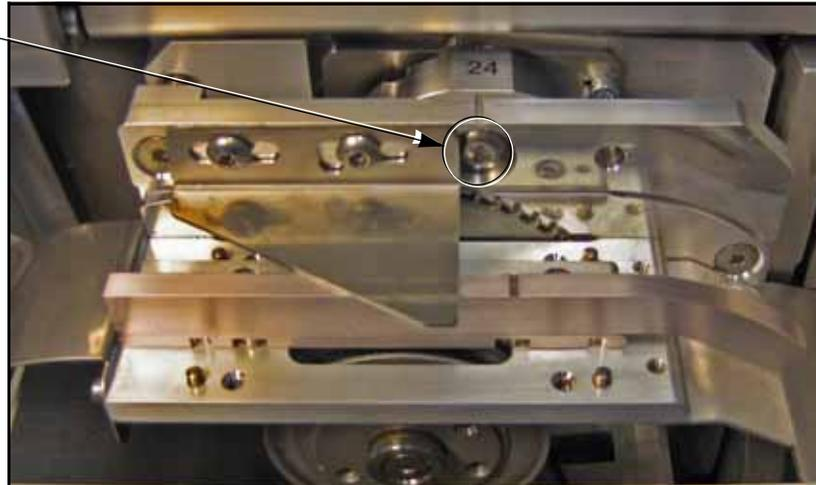
Figure 4-4—Location of Tape-In Module Position Locking Screw (circled). (Base Mounting Screws are Hidden.)
