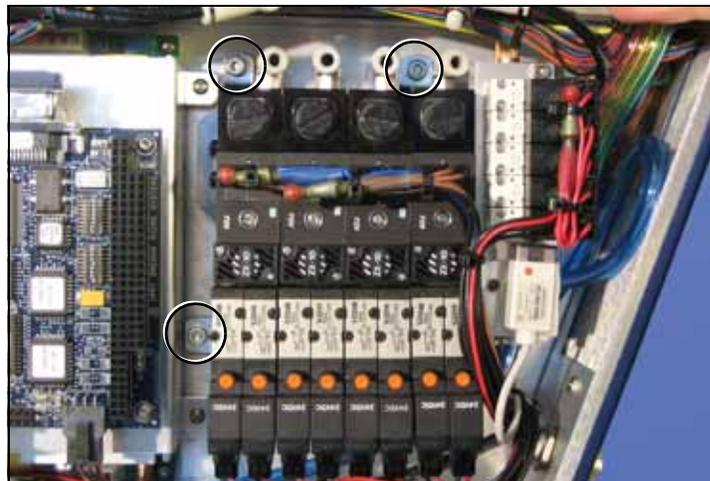
Figure 4-13—Pneumatic Module fastener locations. The Probe Vacuum Tubes have been Disconnected.
