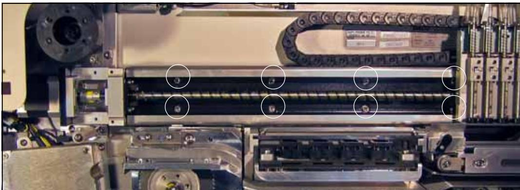
Figure 4-54—Linear Stage Module screw locations (circled). (The Conveyor Module would not be in place at this time.)
