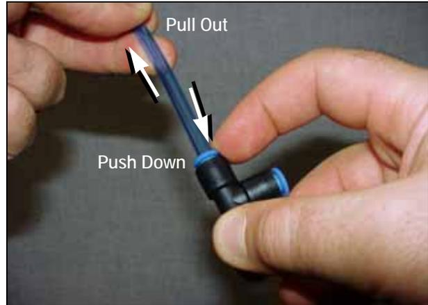
Figure 4-10—Disconnecting a Pneumatic Tube from the One-touch Connector
