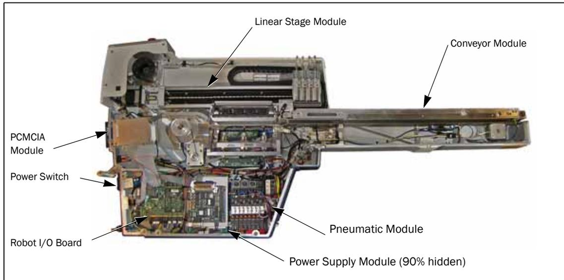
Figure 4-58—Parts in the Self-Service Spares Kit; RoadRunner3
