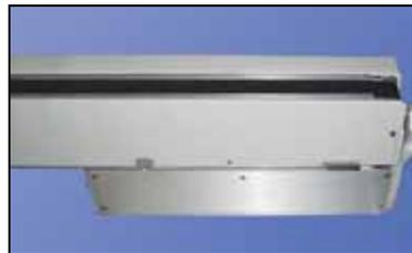
*If the SMT Adapter is not attached to the RoadRunner3, contact Data I/O support— attaching it requires removing the Conveyor Cover.*
