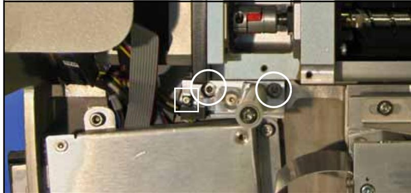
Figure 4-17—The Cover Tape Tensioner with mounting screws (circled) and Sensor screw (boxed).
