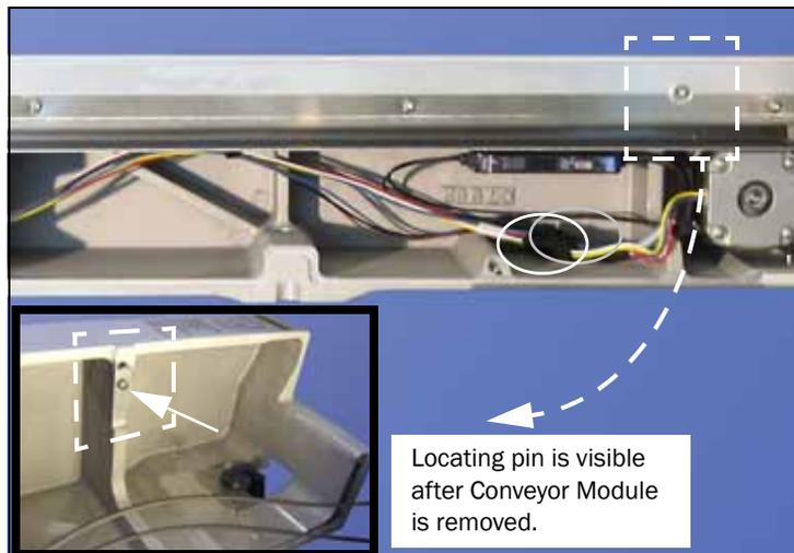
Figure 4-19—Conveyor Wire Connector Locations (Circled).
