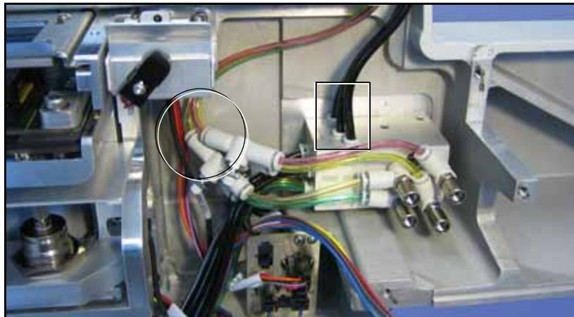
*Figure 4-52—Air tubes from the Linear Stage must be disconnected: four black tubes (boxed) and four colored tubes (circle). The Conveyor Module has been removed, but wires are not disconnected—the wires can be seen descending from the chassis.*
