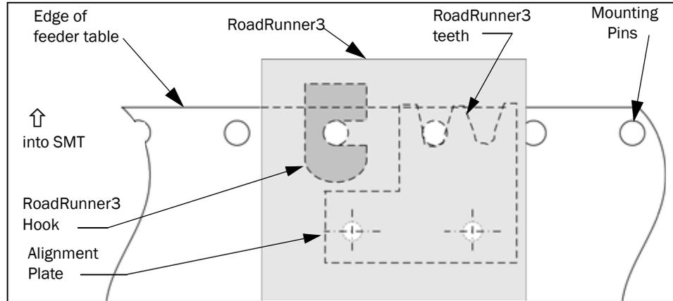
Figure 2-13—Hook Location Relative to RoadRunner3 Placement. Top View
