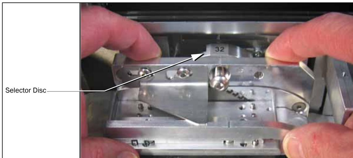
Figure 3-9—Pull the adjustment assembly out for access.
