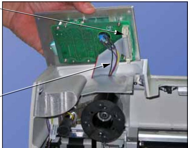
Figure 4-31—Location of Connector on the Control Panel.
