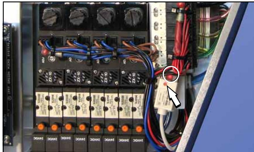
*Figure 4-14—Adjusting the Low Pressure Sensor on the Pneumatic Module. The arrow points to the adjustment screw. The LED is circled.*
