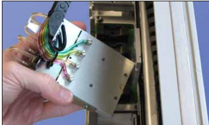
Figure 4-40—The four fittings on the back of the PNP Head. (The Head has been unbolted from the Linear Stage).
