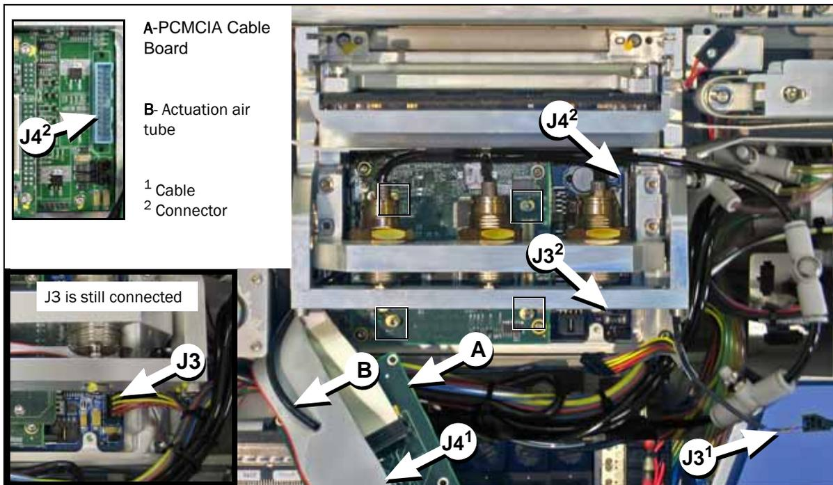
Figure 4-42—PCMCIA Cable Board [A] has been removed from the Programmer Module (squares). The air tube [B] disconnected. **J3** and **J4** cables unplugged—see insets for closer views.
