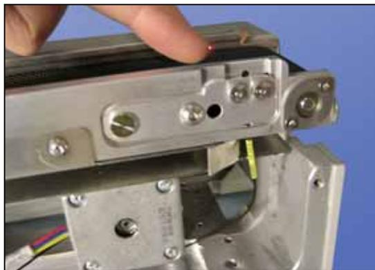
Figure 4-20—Testing the End-of-Belt Sensor (The Conveyor Side Cover need not be removed.)
