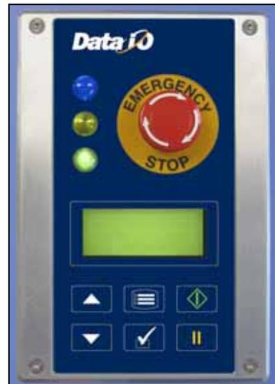
Figure 1-3—The RoadRunner3 Control Panel and Display Screen
