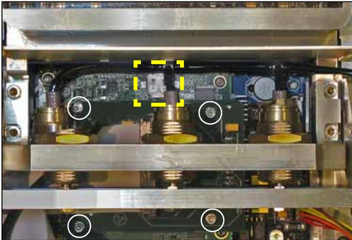
Figure 4-46—The Programmer with Ribbon Cable J4 disconnected. The shiny NVRAM Battery is boxed. PCMCIA Board screws are circled.
