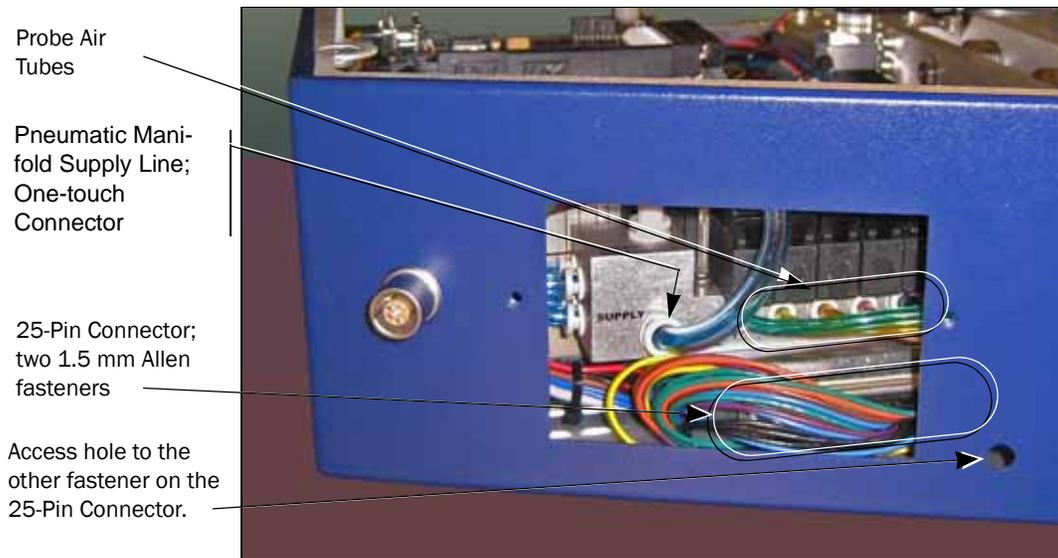
Figure 4-12—Location of the Pneumatic Manifold Supply Line and Wiring Connector. (The Pneumatic Access Cover has been removed.)
