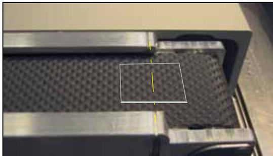
Figure 2-5—Devices center at the pick point marks on the RoadRunner3 conveyor.
