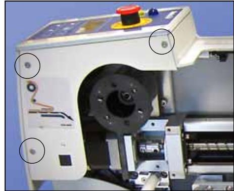
Figure 4-30—Corner Panel Cover with screw locations circled.
