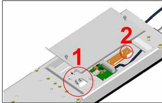
Figure 2-3—The GFI lock screw (M4) is found at (1) when not in use. Move the lock screw to (2) to secure the GFI to the SMT machine.
