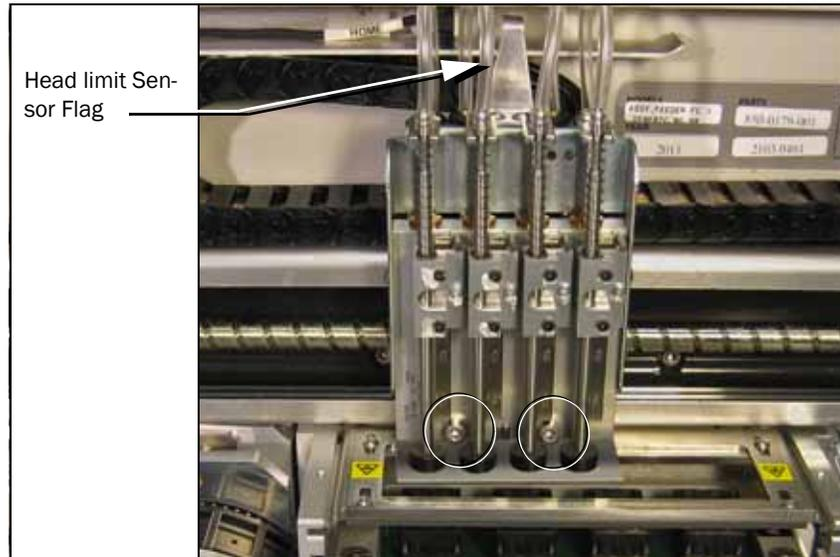
Figure 4-39—The PNP Head Mounting Screws (circled).
