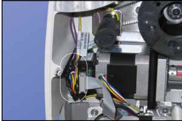
Figure 4-32—Bundle of wires includes the E-Stop Cable connector.
