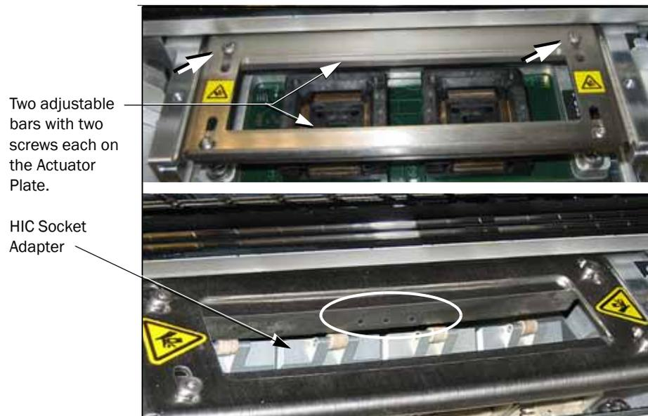
Figure 3-5—Adjustable Actuator Plates: Standard (top) and HIC, identifiable by the three dots, (bottom). Note that the HIC Sockets have rollers.
