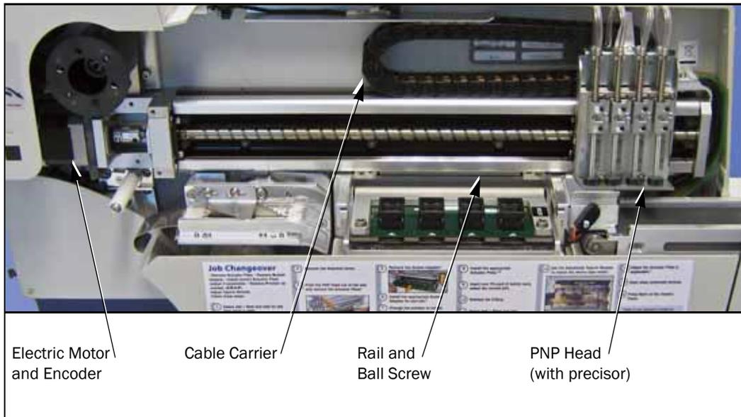
Figure 4-51—The Linear Stage Module.
