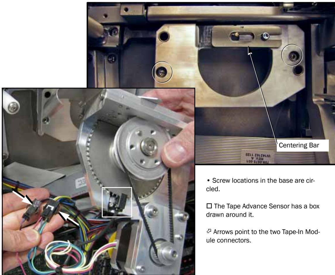
Figure 4-5—The Tape-In Module Base (after the main body has been removed).
