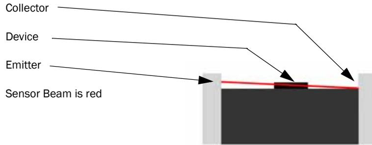
Figure 4-24—A cross-section of the conveyor, looking toward the SMT Assembly Machine.
