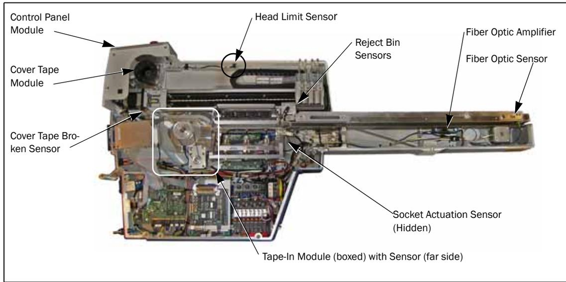
Figure 4-59—Parts in the Supplemental Spares Kit for RoadRunner3
