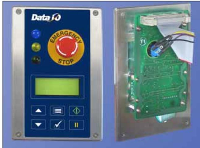
Figure 4-29—Control Panel Module, front and back
