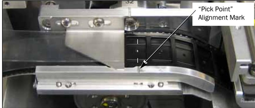
Figure 3-13—Lining Up, by eye, the Device Pocket with the Alignment Mark—alignment need not be exact as shown.
