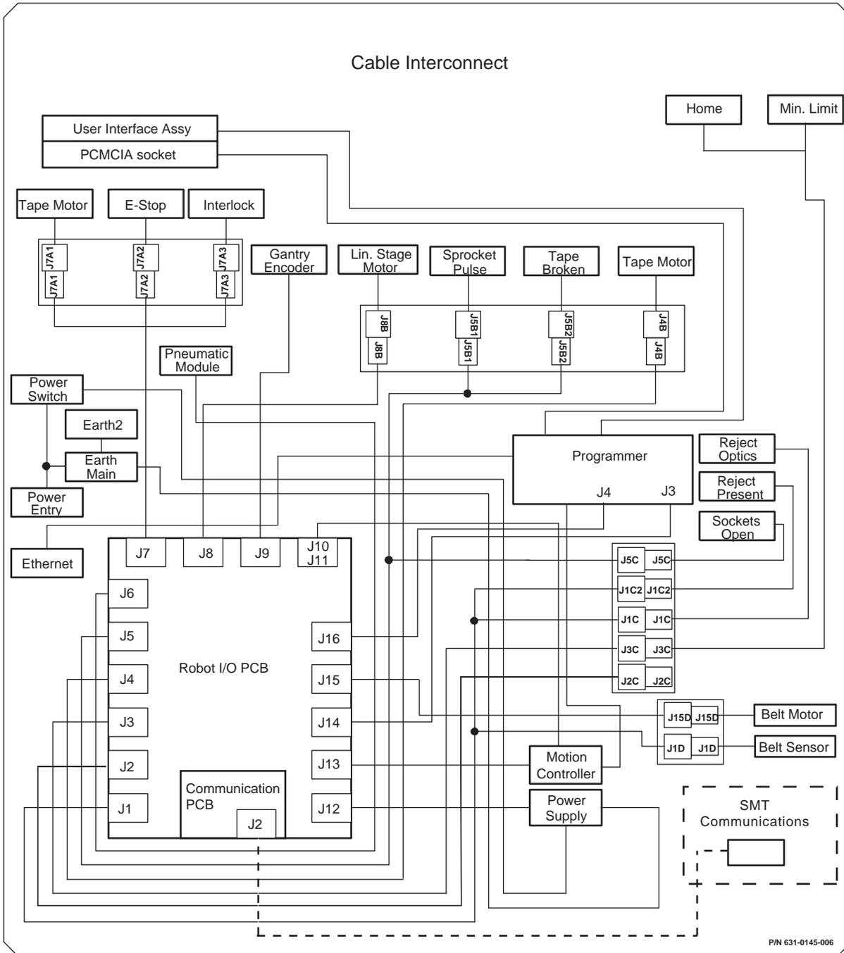
Figure 6-3—Electrical Schematic for all RoadRunner3 Models.
