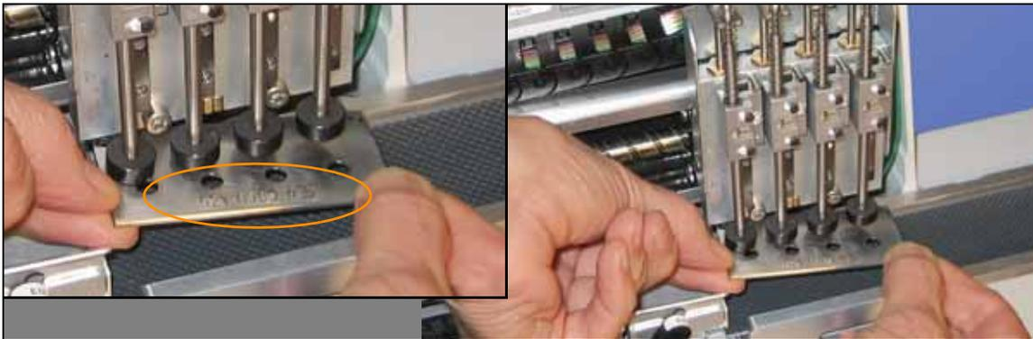
Figure 3-7—Removing the Precisor. The part number is circled.
