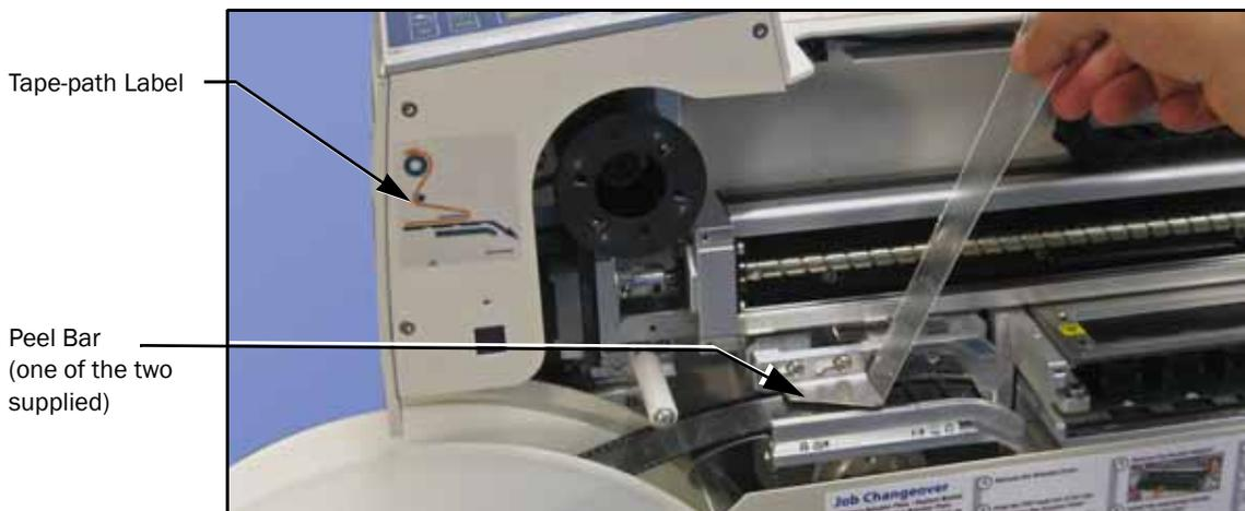
Figure 3-12—Loading device tape. Refer to the label on your unit to determine the tape path and cover tape path.
