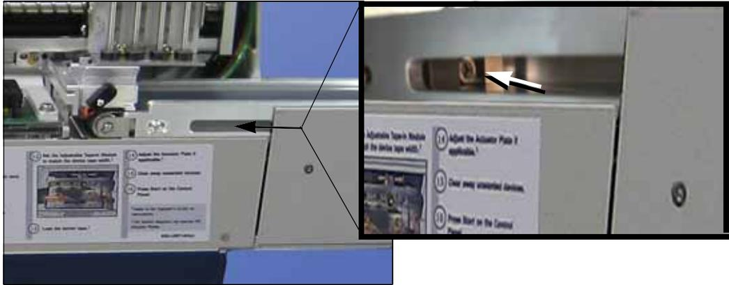
Figure 4-25—The Conveyor tension locking screw (circled) and the Tension Screw (arrow).
