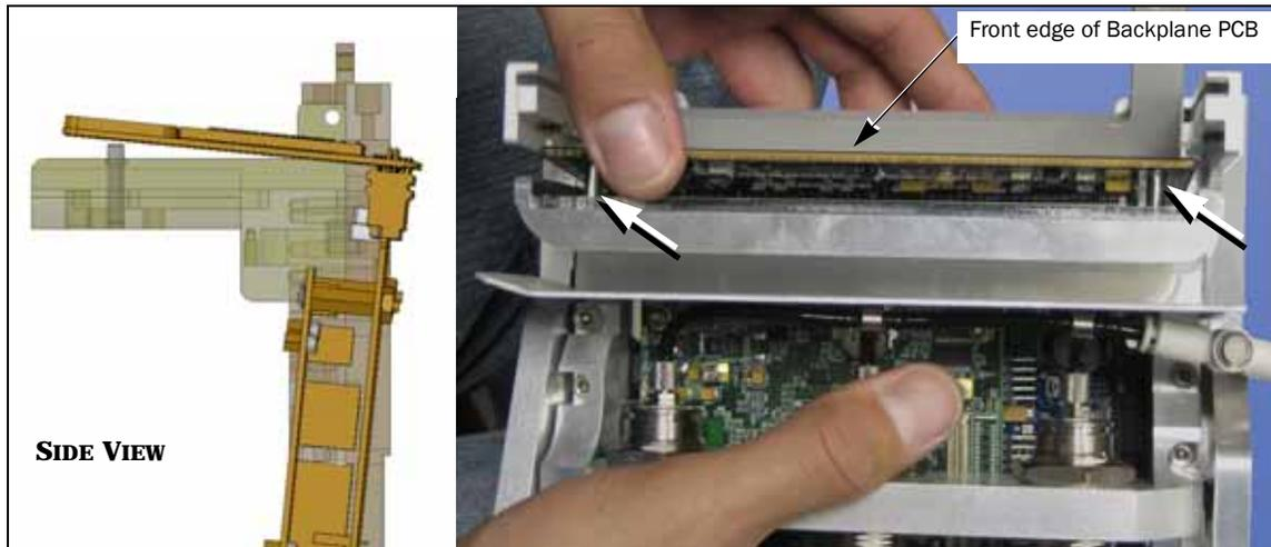
Figure 4-49—Removing the stack of boards off the two dowel pins (arrows) and free of the programmer frame.
