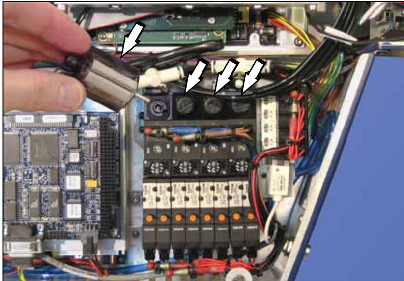
Figure 4-8—Pneumatic Module and Vacuum Filter Locations
