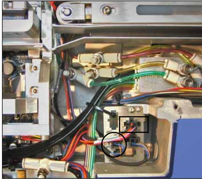
Figure 4-28—Connectors J1C (boxed) and J1C2 (circled).
