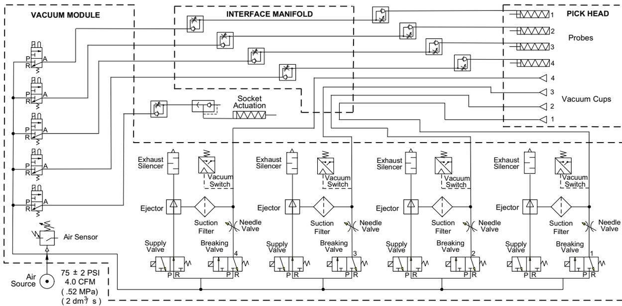
Figure 6-2—RoadRunner3 pneumatic schematic. (Subject to change without notice.)
