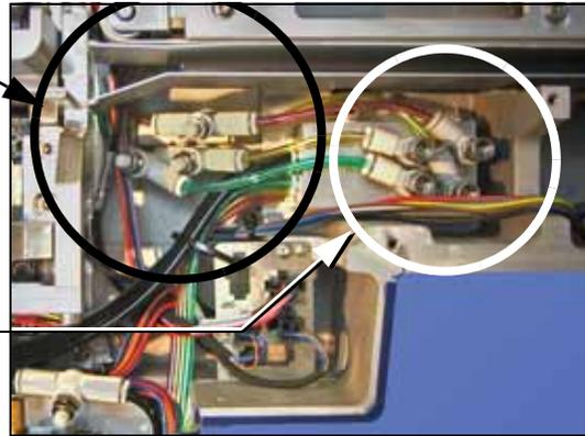
Figure 4-36—The in-line flow controls for adjusting the Probe Speed. Probe numbers are stamped on the manifold.
