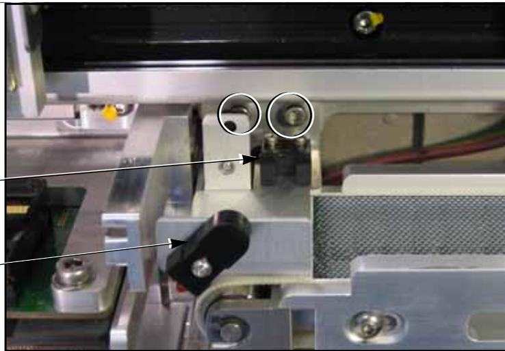
*Figure 4-27—Reject Bin Sensors with Reject Bin Bracket Screw Locations circled. The left screw requires a ball-end hex key. The Reject Bin has been removed.*
