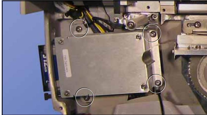
Figure 4-33—PC-card Drive. Four screw locations (circled) require 2.5 mm hex key. The Electronics Covers have been removed.
