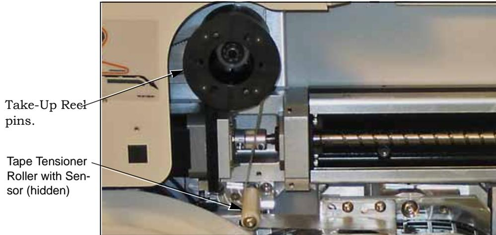
Figure 4-15—Cover Tape Module and the Tape Tensioner
