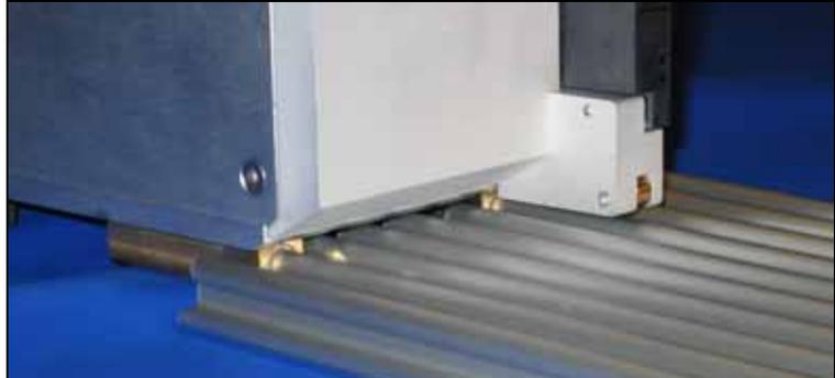
*Figure 2-14—The SMT Adapter on SIPLACE X RoadRunner3 mates with ribs on the Feeder Bank.*
