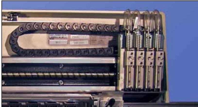
Figure 1-6—Pick and Place Assembly with Precisor.
