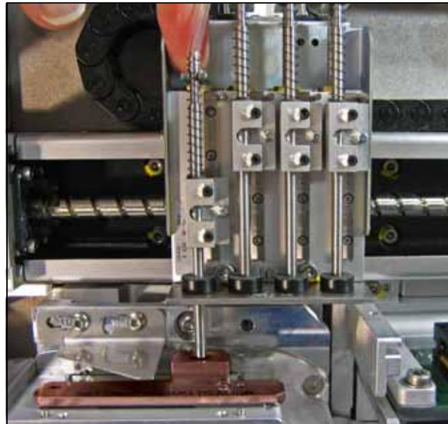
Figure 4-6—The Alignment Tool is installed (copper colored in this image). Push the probe (without tip) down to see if it mates with the slot in the tool.
