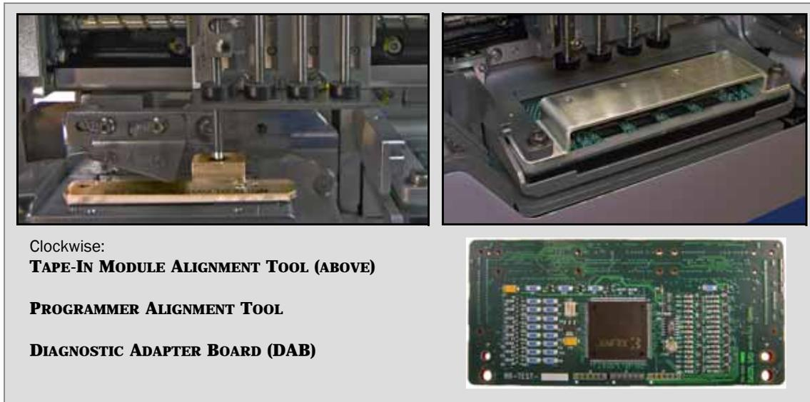
Figure 4-56—Tools in the Alignment Kit; RoadRunner3
