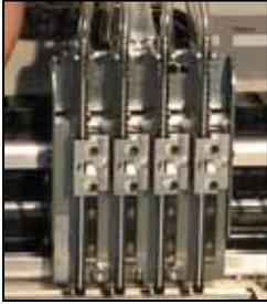
The PNP head Module contains four probes, each with Vacuum Tips. Some parts can be replaced and some probe functions can be adjusted.
