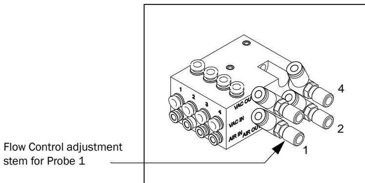
*Figure 4-35—Probe Control Manifold (Adjustment stems require a flat screwdriver for adjustment.)*
