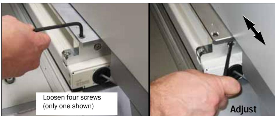
Figure 2-6—Adjusting the pick point.
