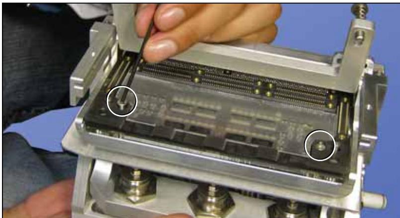
Figure 4-47—Removing the Backplane board from the programmer frame. Screws are circled.
