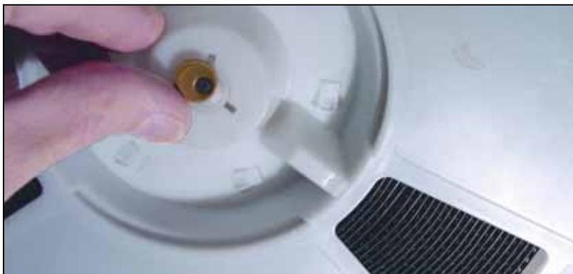
Figure 3-11—Locking a Reel onto the Spindle by rotating the brass button.
