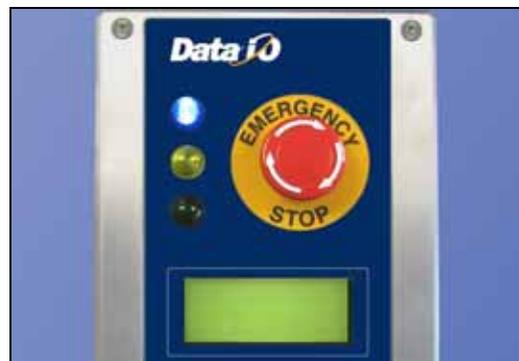
Figure 1-7—Emergency [movement] Stop Button
