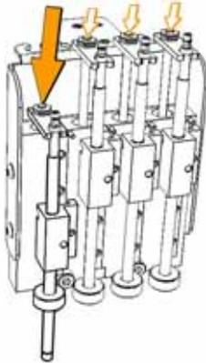
mounting screws (two upper screws) before each attempt to adjust the Programmer Alignment Screws.
