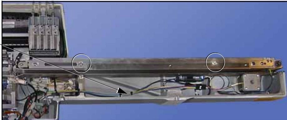
Figure 4-18—Location of wires and mounting screws (circled) on the Conveyor Module (covers removed).
