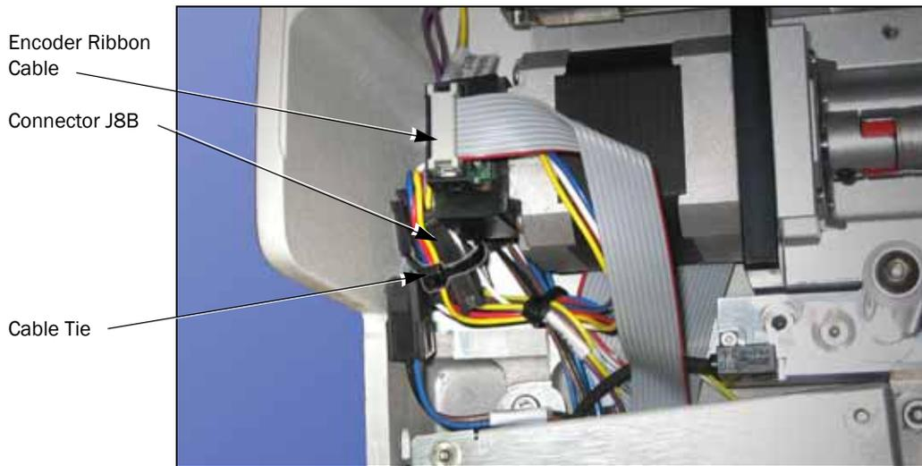
Figure 4-53—Two wire connectors must be unplugged from the Linear Stage Module.
