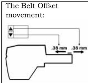
The **Offset** command in the **Belt** menu allows adjusting the device position to accommodate the SMT pick head in the event that centering the device at the pick point (via the **Measure Device** command) is undesirable. Scroll to, and select, [✓] **Robot Diags** > **Belt** > **Offset**. Push the *Up* or *Down Arrow* once to adjust and wait for the belt to adjust the position. Press *Menu* to record and exit the **Offset** command.
