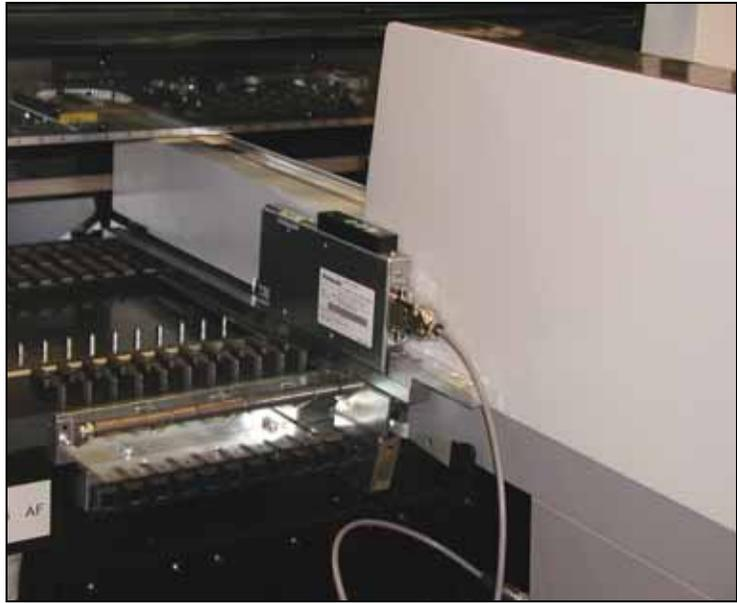
*Figure 2-11—RoadRunner3 is mounted and the Communication Cable is plugged into the Panasonic Host Feeder unit. (RoadRunner model is shown for an example.)*
