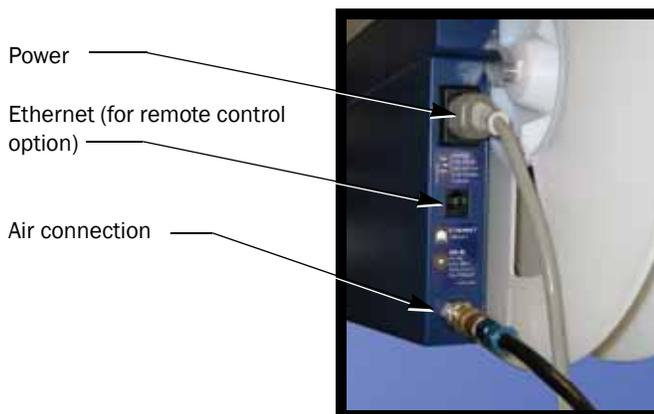
*Figure 2-16—RoadRunner3 facility connection points on the 'Facilities Panel.' For most models, the communication connection is on the far side (not visible here).*
