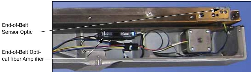
Figure 4-21—Reteaching the End-of-Belt Sensor.
