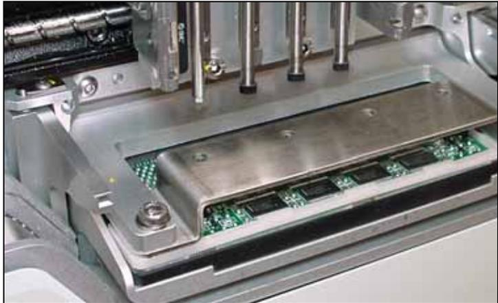
Figure 4-44—The Programmer Module Alignment Tool Installed on the Programmer in place of a Socket Adapter. (PROBE TIPS MUST BE REMOVED PRIOR TO ALIGNMENT PROCEDURE.)
