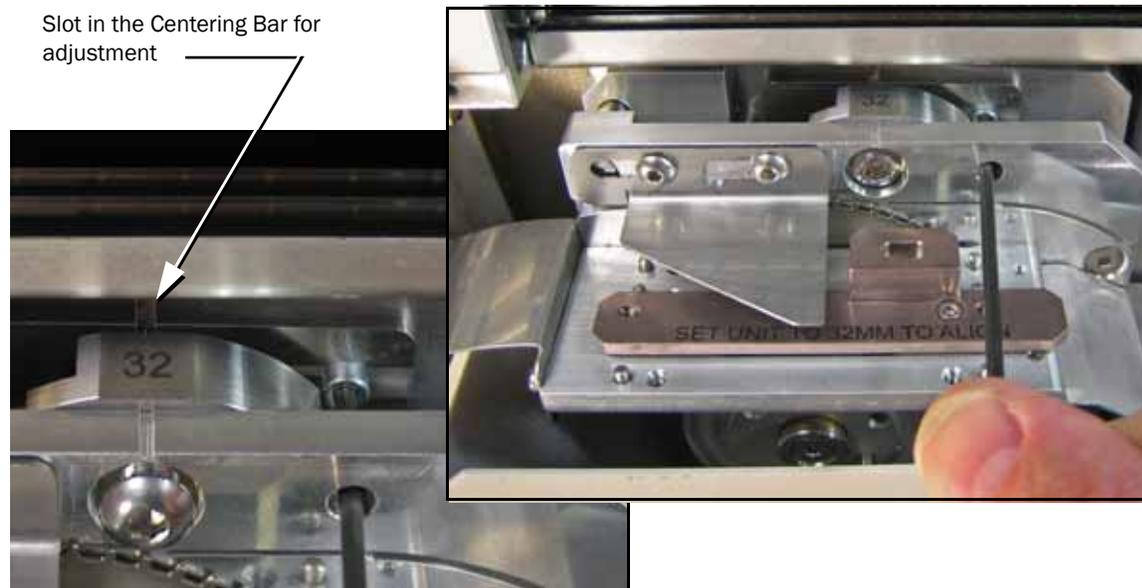
*Figure 4-7—Adjusting the Tape-In Module: loosening the Centering Bar screw. The Centering Bar Adjustment slot is visible.*
