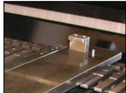
Figure 2-9—The Panasonic Feeder Bank Adapter has a hook and a dowel pin.
