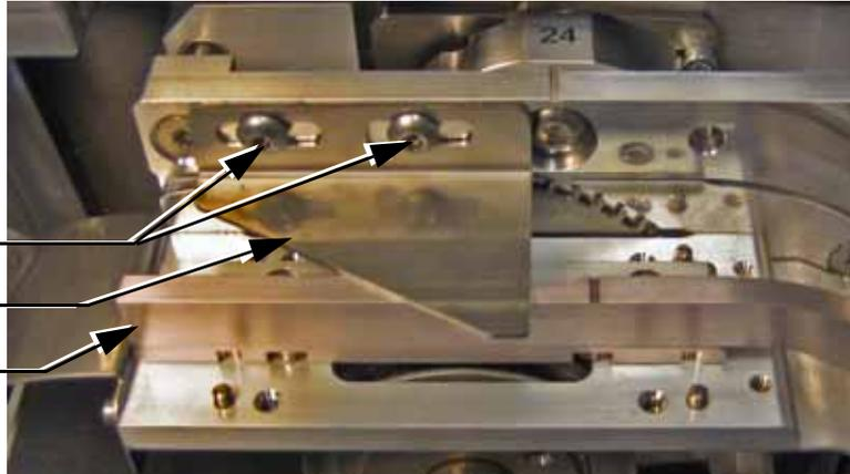
Figure 3-10—Front Track is installed at the 24 mm location to match the Selector Disc setting.
