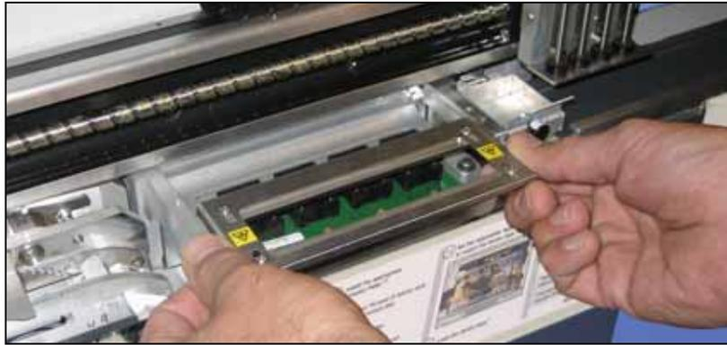
Figure 3-6—Changing the Actuator Plate
