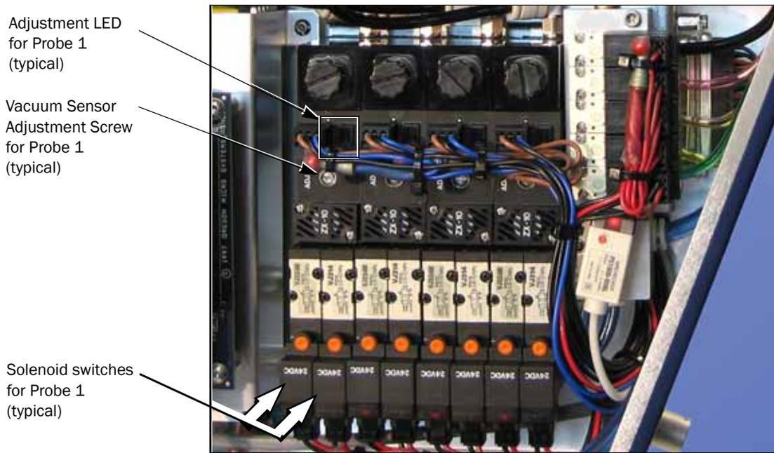
Figure 4-38—Pneumatic Valve Block. When the vacuum for Probe 1 is enabled, the two small LEDs on the solenoids (white arrows) for Probe 1 will be unlit.
