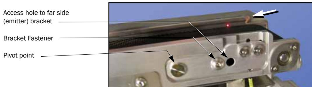
Figure 4-23—The End-of-Belt brackets. Only the tip of the far side bracket is visible (arrow).
