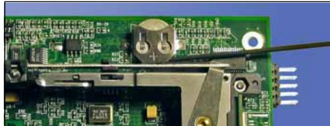
Figure 4-50—Pushing the battery up out of the clip. (Your RPX-Lite board may not look like this.)
