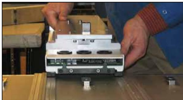
*Figure 2-2—Install the Feeder Bank Adapter onto the SMT Machine separately.*
