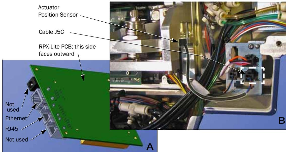
*Figure 4-43—A = The RPX-Lite PCB is part of the programmer. B = Cable Interconnect Panel with the Cable JC5 and Sensor highlighted.*
