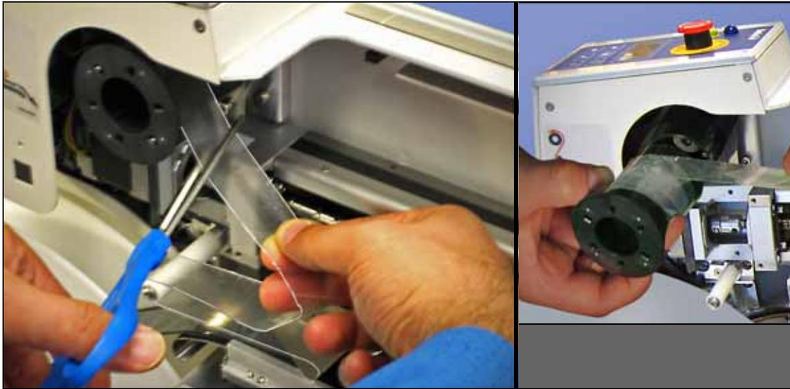
Figure 3-15—Removing the Cover Tape Take-up Reel.
