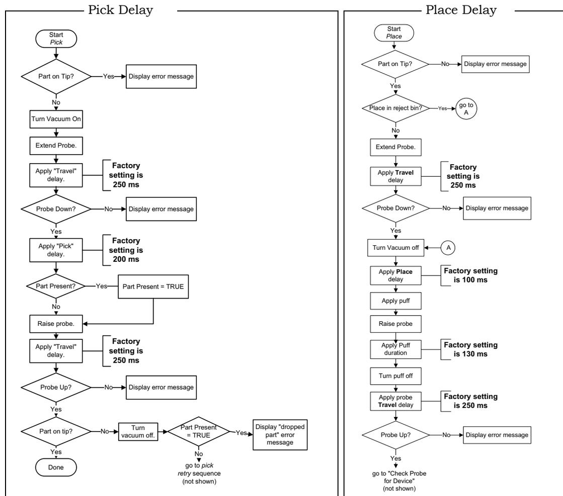
Figure 4-37—Pick and Place Delay Flow Charts
