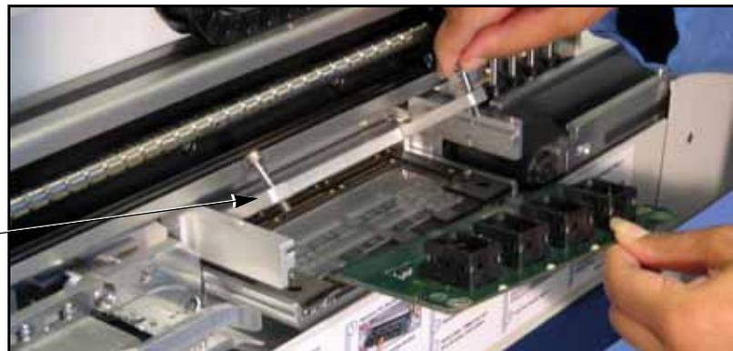
Figure 3-4—Removing the Socket Adapter
