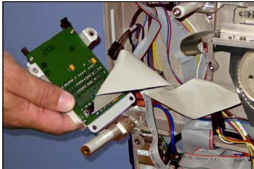
Figure 4-34—PC Drive Ribbon Cable is attached to the back of the drive.
