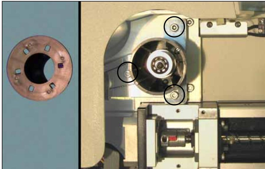
*Figure 4-16—Location of the Cover Tape Module Mounting Screws (circled). The Take-Up Reel has been removed. The Control Panel Cover has not yet been removed.*
