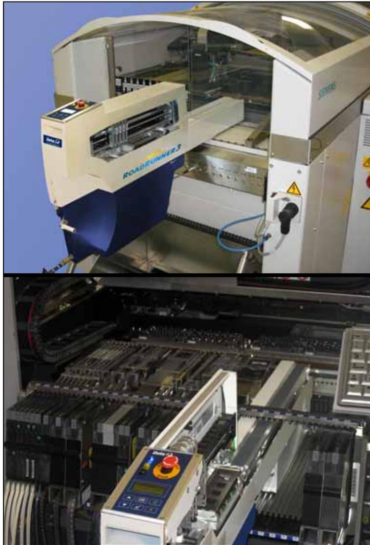
Figure 1-2—RoadRunner3 installed on an SMT Machine (top) and RoadRunner3 on a SIPLACE-X SMT (bottom).
