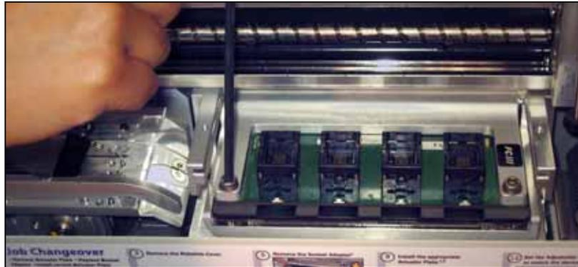
Figure 3-3—Unscrewing the Screws Securing the Socket Adapter
