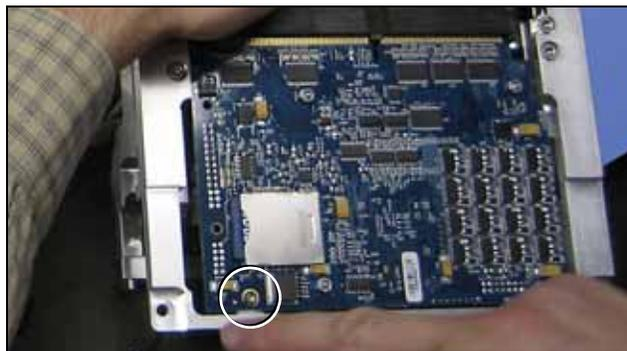
Figure 4-48—The back side of the Waveform board. The attachment screw is circled.
