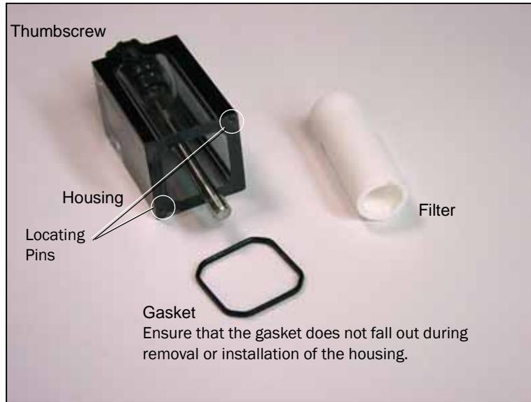
Figure 4-9—Vacuum Filter Components
