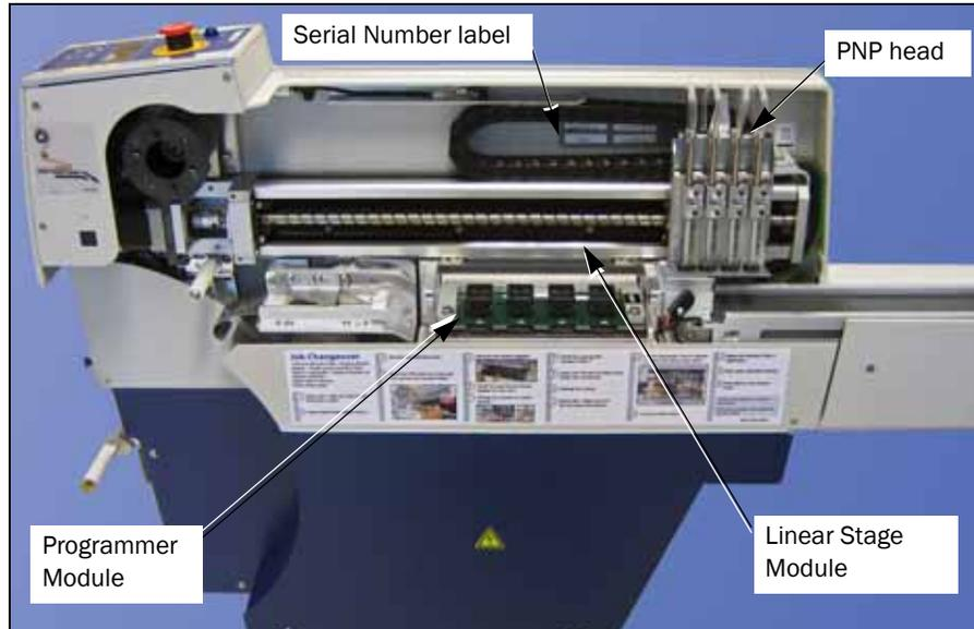
Figure 1-5—Parts of RoadRunner3. The Serial Number label is on the casting.
