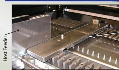
Install the Feeder Bank Adapter, lining it up with a slot and sliding fully forward. Tighten the set screw. Slide the Host Feeder onto the slot immediately left of the adapter, as far as it will go.
