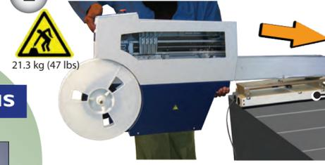
Slide the nose of RoadRunner3 under the hook so the teeth engage the pin next to the hook. Lower RoadRunner3 so the hole under the conveyor engages a second pin.
