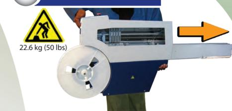
Lower the nose of the conveyor into the beginning of a slot on the Feeder Table and slide fully forward until it locks into place.
