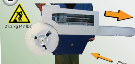
Slide the nose of RoadRunner3 under the hook so the teeth engage the pin next to the hook. Lower RoadRunner3 so the hole under the conveyor engages a second pin.
