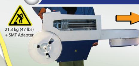
Align the SMT adapter grooves with ribs on the Feeder Bank and slide fully forward.
