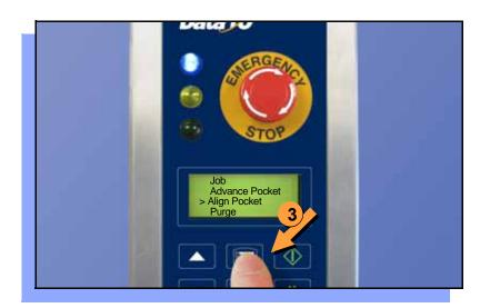
NOTE: If you pass the mark by more than one Up Arrow increment (2 mm), remove the device and use the next pocket. Always approach the mark with the tape traveling forward.
