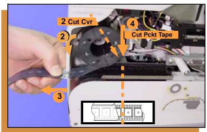
If the tape jams, an error message displays and the blue lamp illuminates.
