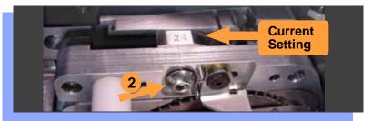
If you have an Adjustable Tape-In Module, you may need to adjust the tape width.
