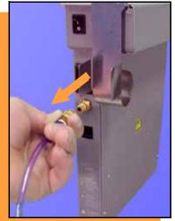
Connect to a grounded power source using a cable with a standard IEC 320 plug.
