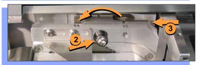
RoadRunner XLF comes with an Adjustable Tape-In Module for 32 mm and 44 mm device tape. A notch points to an etched number indicating the current setting.
