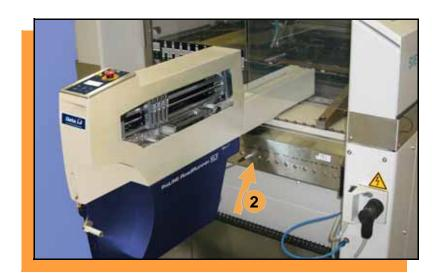
2. Similarly orient and plug the other end of the cable into the SMT feeder table. Use the socket that corresponds with the track that RoadRunner is mounted on.
