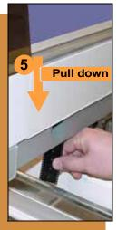
If the tape jams, an error message displays and the blue lamp illuminates. To clear the tape path:
