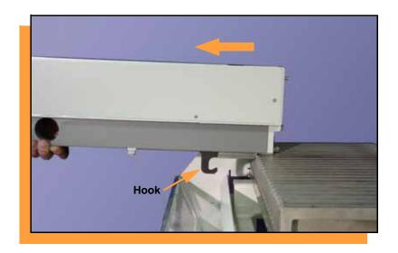
3. Lower RoadRunner. Its own weight will cause it to latch to the feeder bank.
