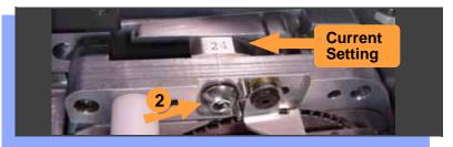
If you have an Adjustable Tape-In Module, you may need to adjust the tape width.
