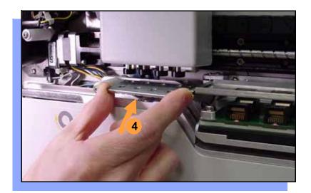
4. When inserting the new precisor, make sure that the part number faces up and that the small holes near the precisor edge fit over the dowel pins on the PNP head.
