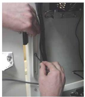
Figure 1-46—Tighten three screws holding new door support
