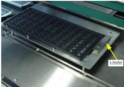
Figure 1-40—L bracket secures tray in position on static tray platform
