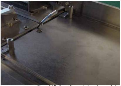
Figure 1-37—Route fiber optic through access hole
