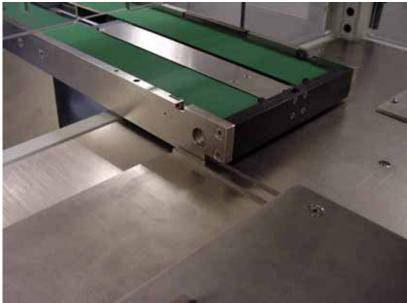
Figure 1-63—Align side rails of TF30 with slots on mount plate and slide forward
