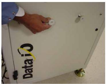
Figure 1-62—Adjust TF30 supports fully inboard
