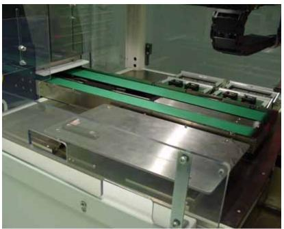
Figure 1-66—TF30 Tray Feeder and static tray
