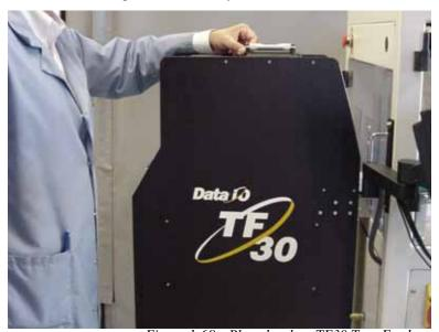
Figure 1-68—Place level on TF30 Tray Feeder
