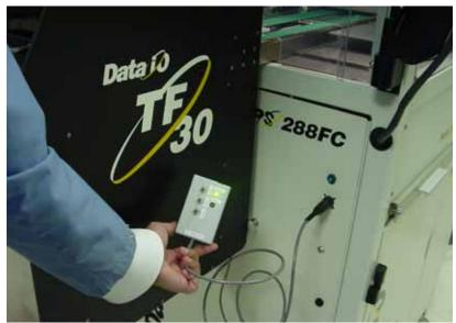
Figure 1-71—Plug in TF Simulator
