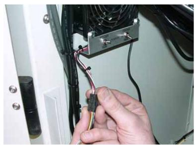
Figure 1-50—Connect door wire harness to switch panel harness
