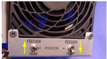
Figure 1-28—Set switch panel to match tray configuration
