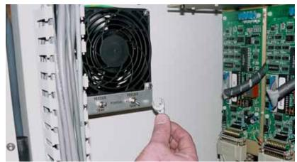
Figure 1-14—Install switch panel
