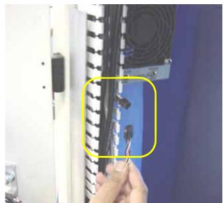
Figure 1-15—Connect door wire harness to switch panel harness
