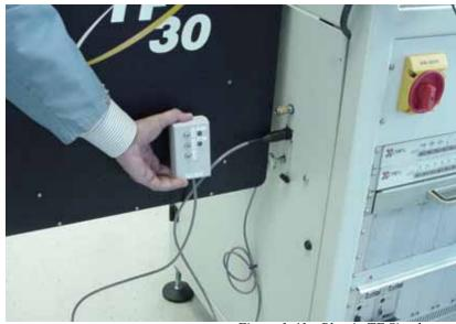
Figure 1-41—Plug in TF Simulator
