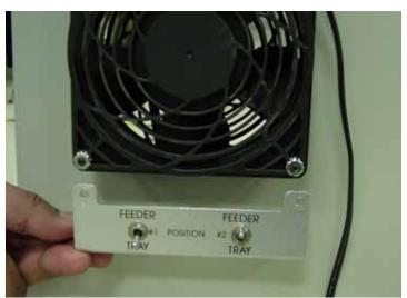
Figure 1-44—Install switch panel to exhaust fan bolts
