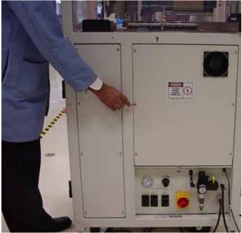
Figure 1-43—Loosen screws on back panel
