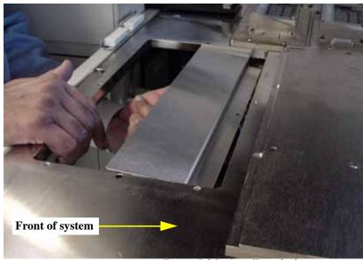
Figure 1-26—Installing the bottom cover
