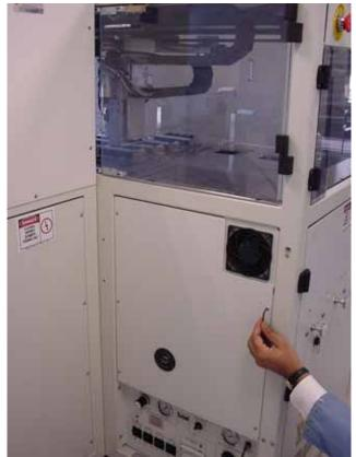
Figure 1-6—Remove back panel (shown with Option Bay)
