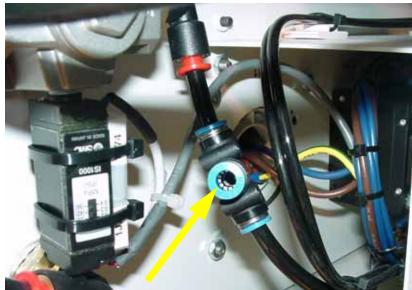
Figure 1-17—Insert air tube from door into fitting as indicated by arrow
