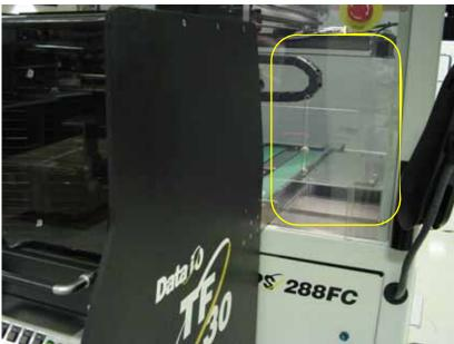
Figure 1-67—Unused slider is closed
