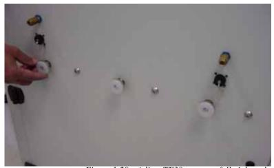
Figure 1-29—Adjust TF30 supports fully inboard
