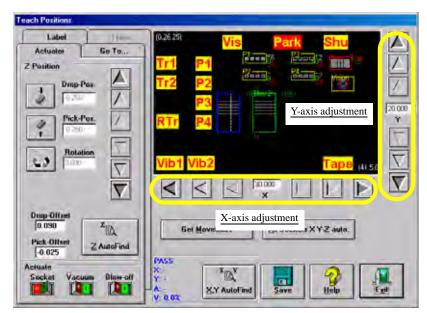
Figure 1-9—Adjustment arrows for X- and Y-axes
