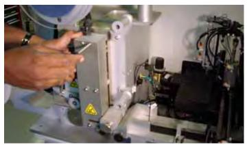
Figure 2-22—Installing heat seal unit
