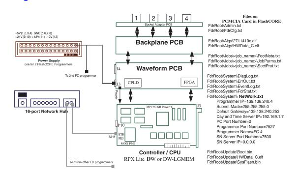
*Figure 4-2—Internal structure of FlashCORE programmer*
