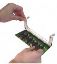
Figure 3-25— Lift the Socket Adapter
