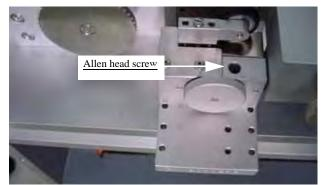
*Figure 2-23—Adjusting width of pressure seal unit*
