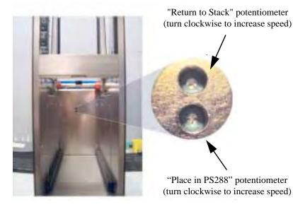
Figure 5-79—Conveyor speed potentiometers
