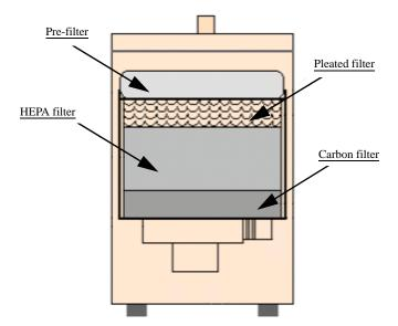
Figure 5-24—Laser vacuum filter locations
