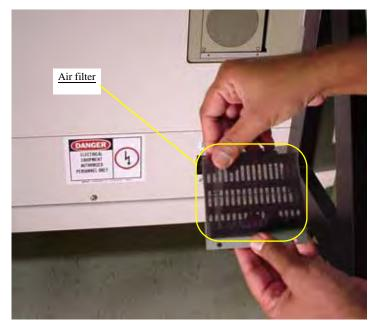
Figure 5-22—Replace air filter
