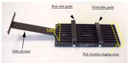
Figure 2-7—Input tube loader platform
