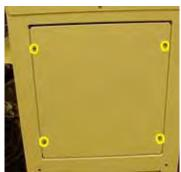
*Figure 5-17—Side laser housing panel screw locations*
