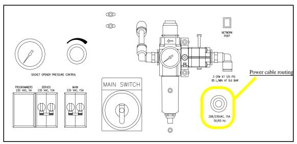
Figure 2-2—Power cable routing through input panel
