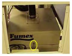
Figure 5-28—Filter system spring clip
