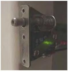
*Figure 1-12—Laser safety interlock*
