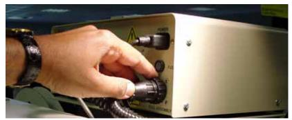
Figure 2-25—Power cord in tape output controller
