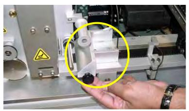
Figure 2-29—Remove sensor clamp block
