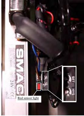
Figure 5-30—Vacuum sensor light. SET and HYS adjustment screws
