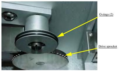
Figure 5-77—Idler pressure wheel and O-rings
