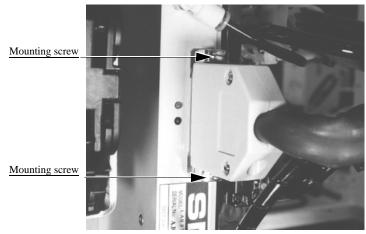
Figure 5-10—PNP head mounting screws
