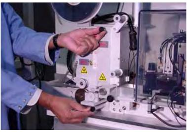
Figure 2-24—Installing pressure seal unit
