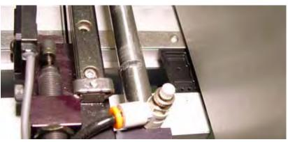
Figure 2-19—Carrier tape threaded into track
