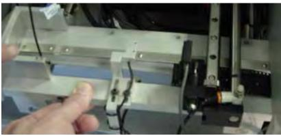
*Figure 2-20—Adjustable Loading Track*
