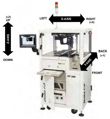
Figure 1-1—PS288 motion axes
