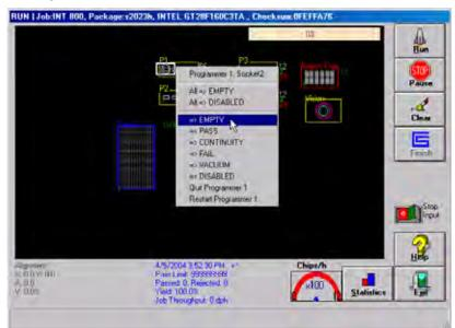
Figure 3-21—Re-enabling a single socket
