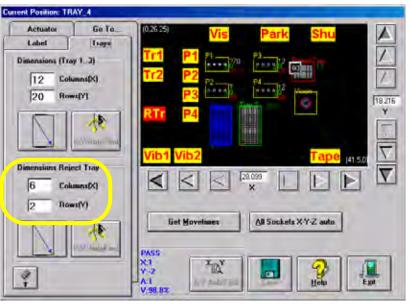
Figure 3-57—Setting number of devices sent to reject tray
