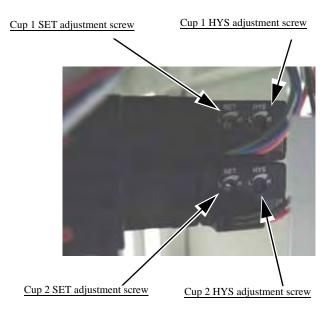
Figure 5-33—Cup 1 and Cup 2 vacuum generator adjustments
