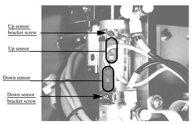
Figure 5-39—Sensors and brackets as viewed from back of PNP head
