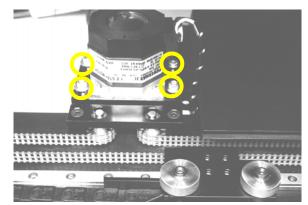
Figure 5-3—Location of four motor mounting screws
