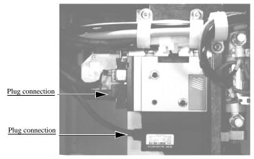
*Figure 5-11—PNP gantry wiring harness plug connections*
