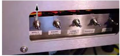
Figure 5-34—Apply Vacuum switch UP
