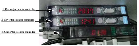
*Figure 5-78—Sensor controllers*
