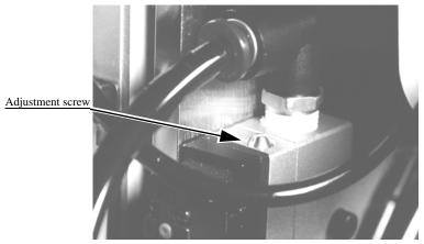
Figure 5-37—Blow-off adjustment screw on vacuum generator
