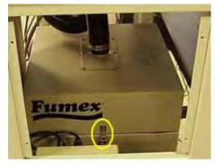
*Figure 5-19—Filter system spring clip*
