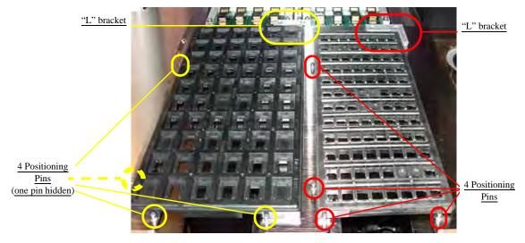
Figure 2-5—Two Static Trays seated with optic sensors (hidden) blocked
