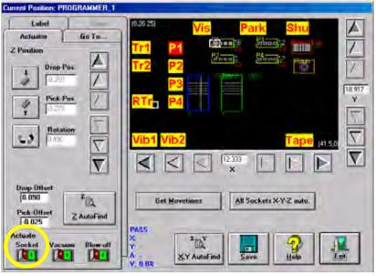
*Figure 5-41—Socket actuator ON*
