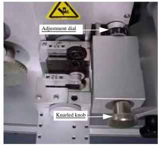
Figure 2-35—Adjusting Cover Tape Guide #3
