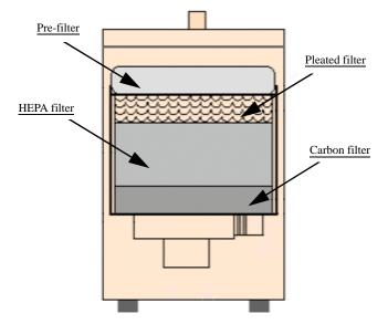
Figure 5-15—Laser vacuum filter locations
