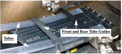
Figure 2-9—Adjust front and rear tube guides
