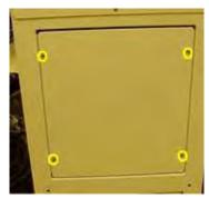
Figure 5-26—Side laser housing panel screw locations
