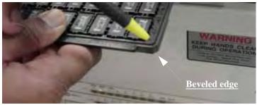
Figure 2-4—Static tray orientation
