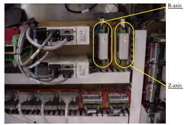
Figure 5-7—Z-axis and R-axis servo motor amps
