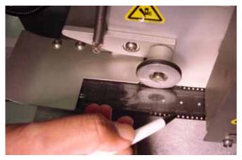
Figure 2-34—Alignment of cover tape over carrier tape
