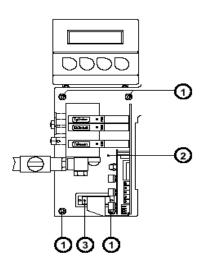
*Figure 2-40—Installing the tamp applicator: 1=screw locations; 2=cover; 3= connector*
