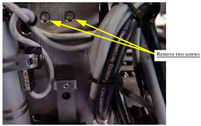
Figure 5-65—Removing upper screws
