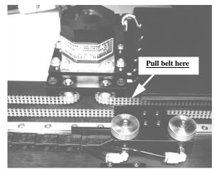
*Figure 5-2—Shuttle belt and motor*
