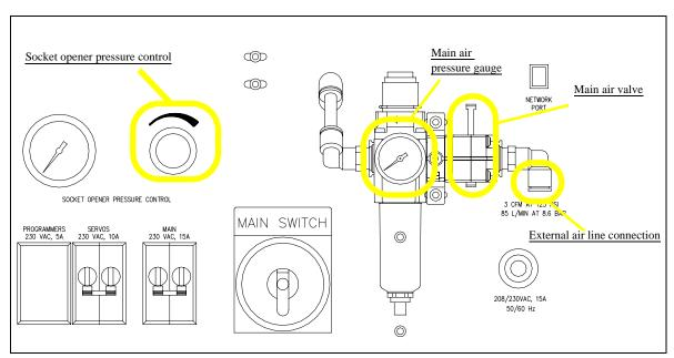
Figure 2-1—Pneumatic input and controls on the input panel
