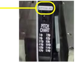
*Figure 2-11—Part number for 32 mm feeder*
