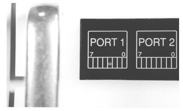
Figure 5-9—I/O Controller LED showing Port 1, Bit 3 is on
