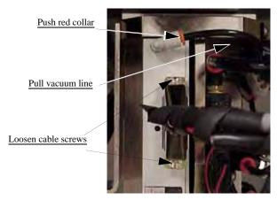
Figure 5-62—Location of vacuum line and cable screws
