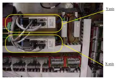
Figure 5-8—Y-axis and X-axis servo motor amps
