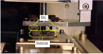
Figure 5-43—Socket actuator ribs contact socket top
