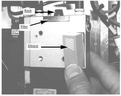
Figure 5-6—Removing the PNP head vacuum filter and silencer
