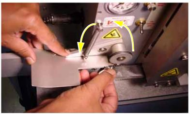
Figure 2-32—Idler Arm and Drive Sprocket
