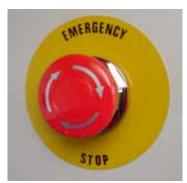
Figure 3-17—Emergency stop (E-Stop) button
