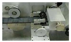
Figure 2-18—Pressure seal unit
