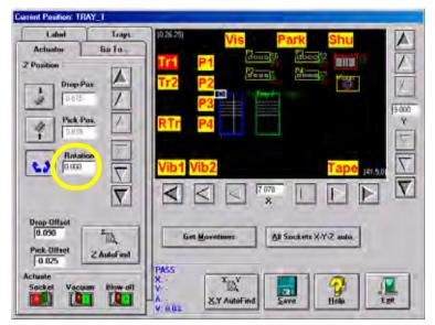
Figure 3-27—Rotation set at 0.000 at Tr1
