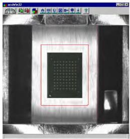
Figure 3-36—Set device search area (red rectangle) around device
