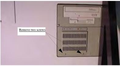
Figure 5-21—Remove screws from Laser Computer filter cover
