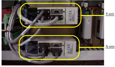
Figure 5-70—Y-axis and X-axis servo motor amps
