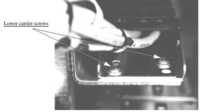
Figure 5-13—Lower carrier screw locations
