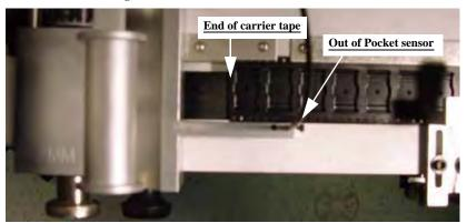
Figure 2-21—Out of Pocket sensor and tape location on the tape output
