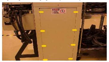
Figure 5-16—Lower back laser housing panel screw locations
