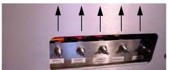
Figure 2-38—Toggle switches should be in UP ("normal") position
