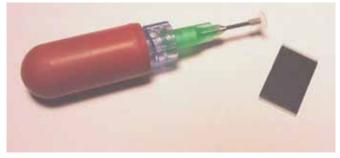
Figure 1-17—Semiconductor device vacuum tool (PN 565-8000-001)
