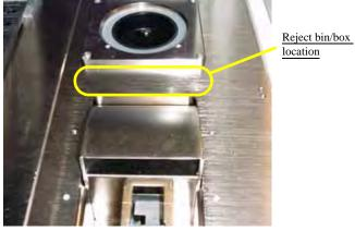
Figure 2-6—Reject bin/box location
