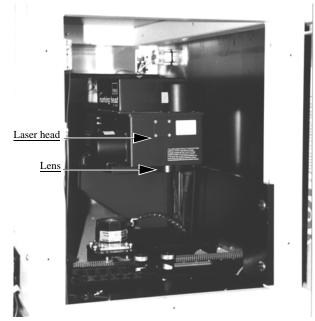
*Figure 5-5—Upper left laser housing with panel removed*
