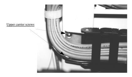
*Figure 5-12—Upper carrier screw locations (one is hidden in this view)*
