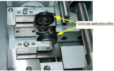
Figure 5-76—Cover tape application rollers
