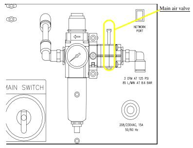
Figure 5-42-Push bar down on main air valve to turn off air
