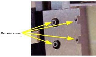
Figure 5-63—Removing four screws
