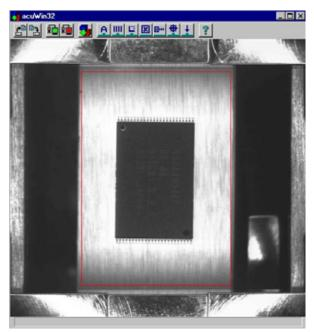
Figure 6-80—Adjust device search area around device
