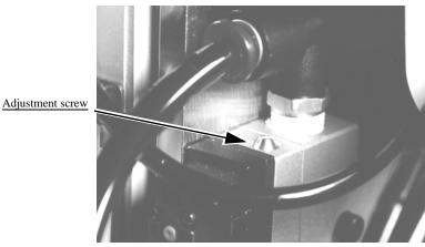
Figure 6-47—Blow-off adjustment screw on vacuum generator
