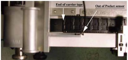
Figure 2-21—Out of Pocket sensor and tape location
