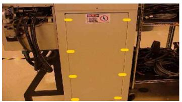
*Figure 6-18—Lower back laser housing panel screw locations*
