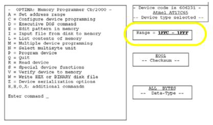
Figure 3-73—Command menu showing address range
