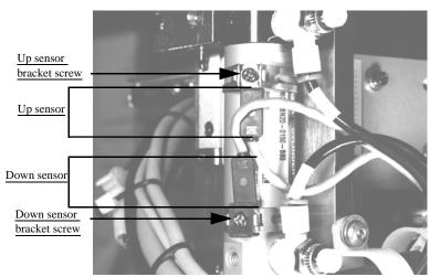
Figure 6-49—Sensors and brackets as viewed from back of PNP head
