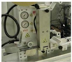
Figure 2-17—Heat seal unit
