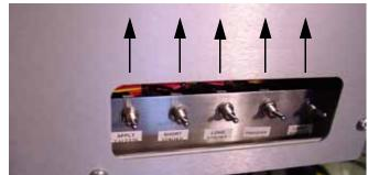
Figure 2-38—Toggle switches in UP ("normal") position
