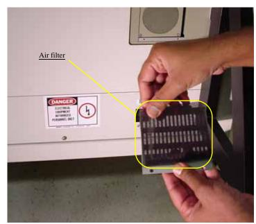
Figure 6-24—Replace air filter
