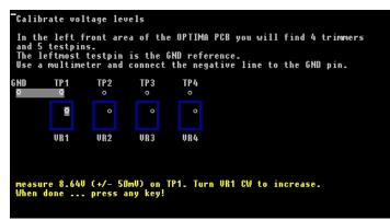
Figure 6-61—TP1 (measure and adjust)
