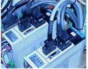
Figure 6-94—Mitsubishi servo motor amps
