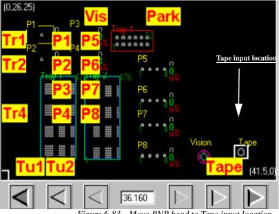
Figure 6-83—Move PNP head to Tape input location
