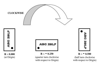
Figure 3-37—R-axis values for CLOCKWISE rotation
