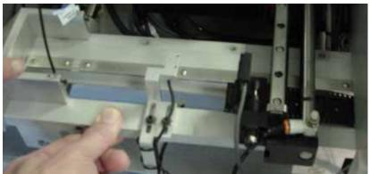
Figure 2-20—Adjustable Loading Track
