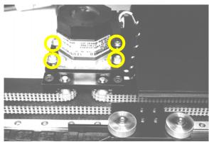
Figure 6-6—Location of four motor mounting screws
