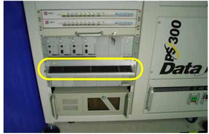
*Figure 6-2—Fan filter drawer*
