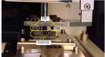
Figure 6-53—Socket actuator ribs contact socket top
