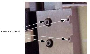
Figure 6-87—Removing socket actuator from guide
