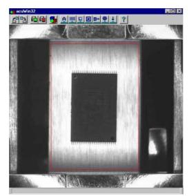
Figure 3-46—Set device search area (red rectangle) around device
