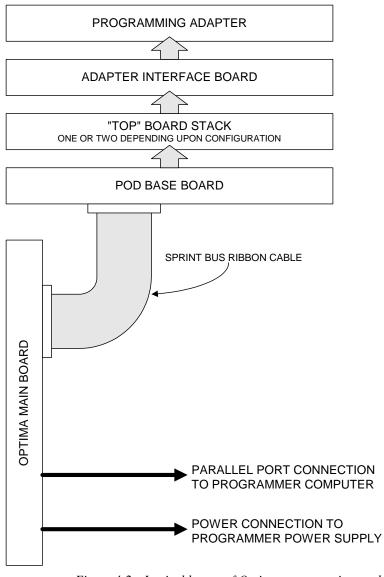
Figure 4-2—Logical layout of Optima programming module
