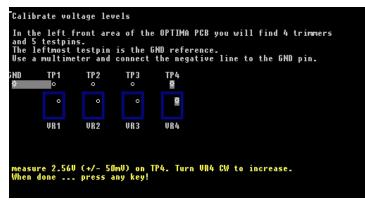
Figure 6-65—TP4 measure and adjust
