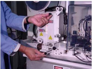
Figure 2-24—Installing pressure seal unit
