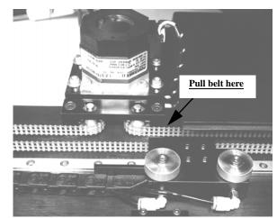
*Figure 6-5—Shuttle belt and motor*
