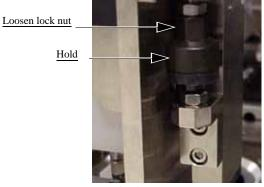
Figure 6-86—Removing air shaft
