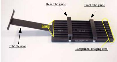
Figure 2-5—Input tube loader
