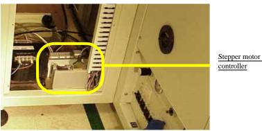
Figure 6-106—Stepper motor controller
