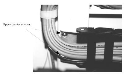
*Figure 6-14—Upper carrier screw locations*
