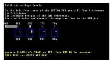
*Figure 6-63—TP2 (measure and adjust)*
