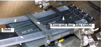
Figure 2-7—Adjust front and rear tube guides
