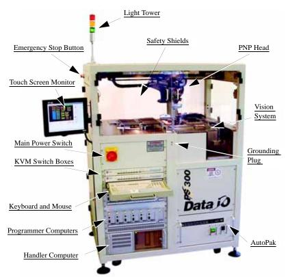
Figure 1-2—PS Series System primary subassemblies
