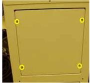
Figure 6-19—Side laser housing panel screw locations
