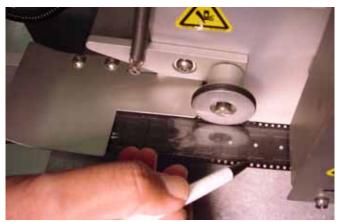
Figure 2-34—Alignment of cover tape over carrier tape
