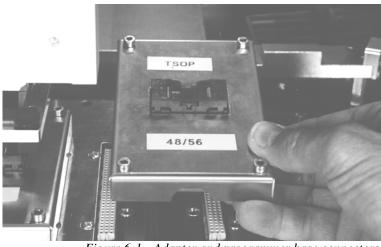
Figure 6-1—Adapter and programmer base connectors
