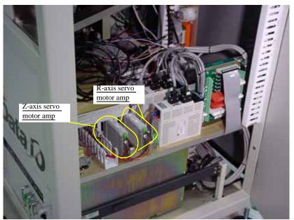
Figure 6-8—Z-axis and R-axis servo motor amps
