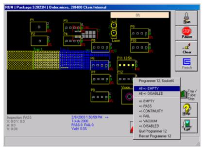
Figure 3-14—Re-enabling programmer
