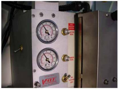
Figure 2-26—Seal pressure control settings
