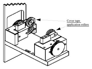
Figure 6-103—Cover tape application rollers
