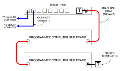
Figure 4-3—Basic PS Series System networking diagram
