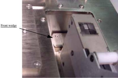
Figure 2-13—Feeder unit sliding under front wedge
