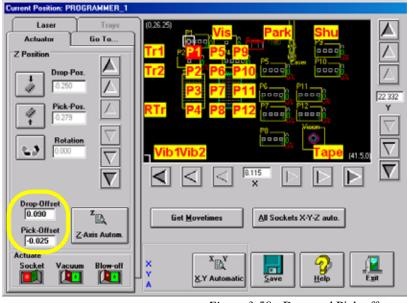
Figure 3-58—Drop and Pick offsets
