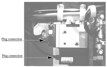
Figure 6-13—PNP robot wiring harness plug connections
