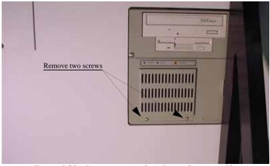
Figure 6-23—Remove screws from Laser Computer filter cover
