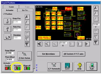
Figure 6-75—Vacuum switch is ON
