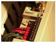
Figure 6-109—Install resistor
