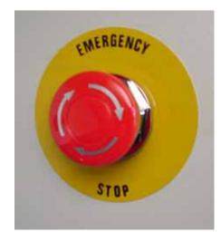
Figure 3-16—Emergency stop (E-Stop) button
