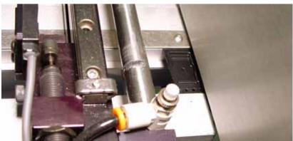
*Figure 2-19—Carrier tape threaded into track*
