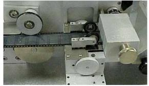
Figure 2-18—Pressure seal unit
