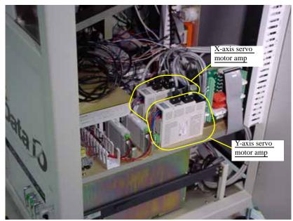
Figure 6-9—X-axis and Y-axis servo motor amps
