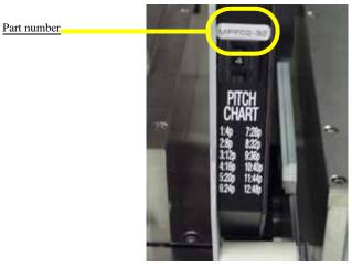
*Figure 2-9—Part number for 32mm feeder*
