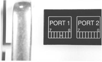
Figure 6-11—AutoPak LED showing Port 1, Bit 3 is on
