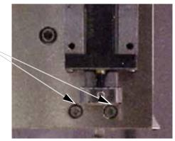
Figure 6-88—Removing lower screws
