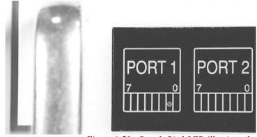
Figure 6-50—Port 1, Bit 1 LED illuminated
