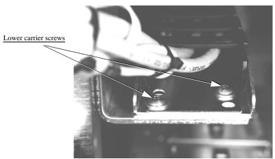
*Figure 6-15—Lower carrier screw locations*
