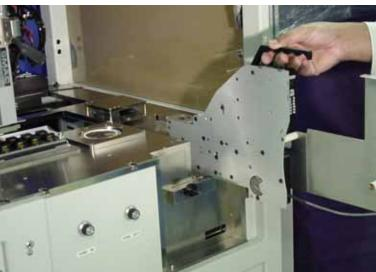
Figure 2-12—Slide feeder unit onto base plate
