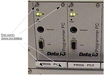
Figure 6-33—Four screws holding Programmer Computer in rack
