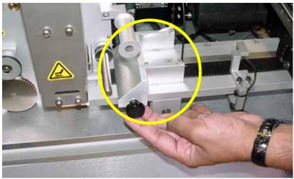
Figure 2-29—Remove sensor clamp block
