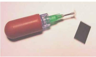
Figure 1-11—Semiconductor device vacuum tool (PN 565-8000-001)
