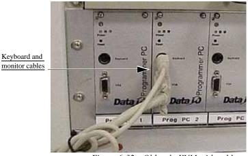
Figure 6-32—Old style KVM with cables
