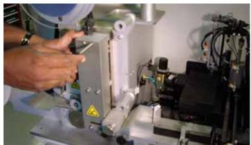
Figure 2-22—Installing heat seal unit
