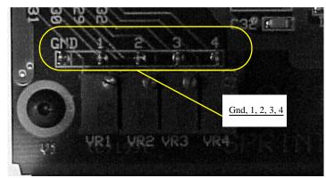
Figure 6-57—Test pins
