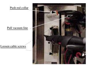
Figure 6-84—Location of vacuum line and cable screws
