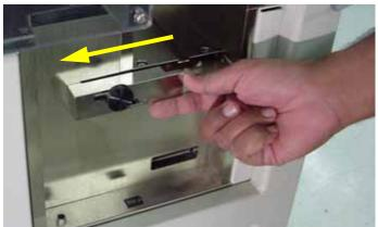
Figure 2-11—Slide lock bar to left
