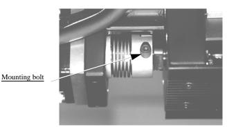
Figure 6-10—Flex coupler mounting bolt
