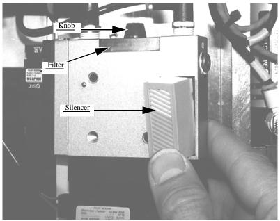
Figure 6-7—Removing the PNP head vacuum filter and silencer
