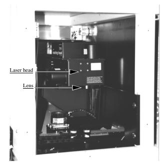
*Figure 6-4—Upper left laser housing with panel removed*
