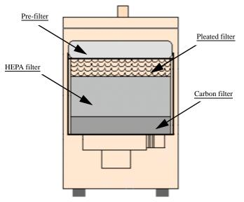
Figure 6-26—Laser vacuum filter locations
