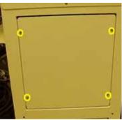
*Figure 6-28—Side laser housing panel screw locations*
