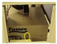
Figure 6-30—Filter system spring clip
