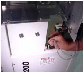
Figure 2-15—Connect interface cable
