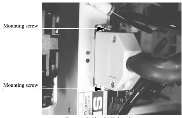
Figure 6-12—PNP head mounting screws
