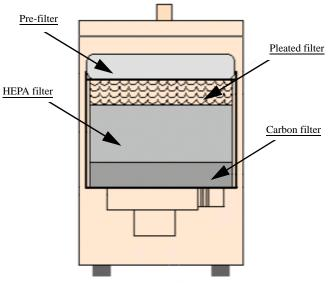
Figure 6-17—Laser vacuum filter locations
