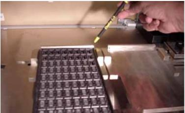
Figure 2-3—Tray seated with optic sensor blocked
