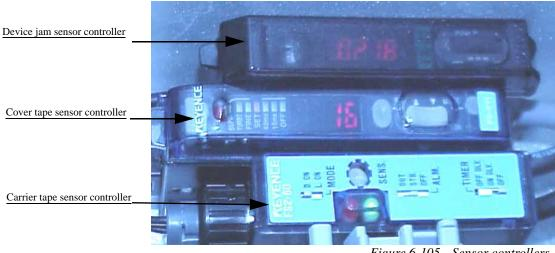
Figure 6-105—Sensor controllers
