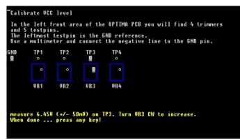
Figure 6-58—TP3 (measure and adjust)
