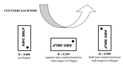
Figure 3-38—R-axis values for COUNTERCLOCKWISE rotation
