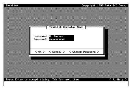
The default operator mode password is **password**. Each operator may create a unique password to replace this default, and can change it by selecting the **Change Password** pushbutton from the login dialog box (see Figure 3-20). Screen prompts guide user through the process.
