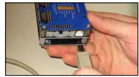
Figure 2-14—Plug the USB Cable into Master IW-300
