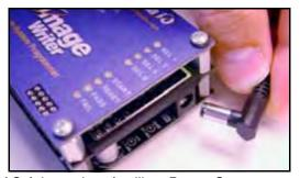
Figure 2-2—Plug AC Adapter into Auxiliary Power Connector
