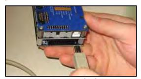
Figure 2-1—Plug the USB Cable into IW
