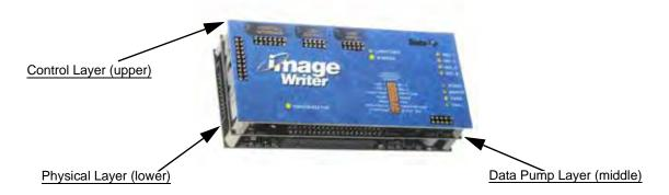
Figure 1-5—IW-300 Showing Three Layers of Hardware
