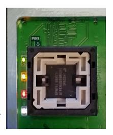
All LEDs will light simultaneously at startup and go off when the startup process is complete.
