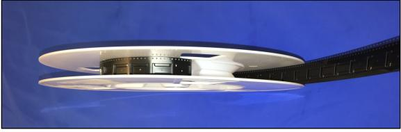
Connect carrier tape to empty tape reel.
