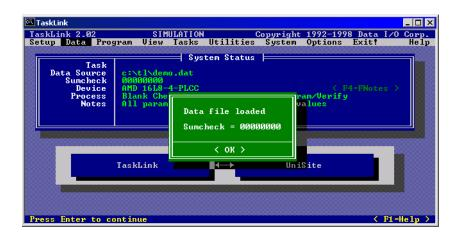
Note: Because TaskLink for DOS is running in Simulation Mode, the checksum displayed is 00000000. When connected to a programmer and loading real data, the checksum will display actual values.
