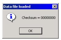
Note: Because TaskLink for Windows is running in Simulation Mode, the checksum displayed is 00000000. When connected to a programmer and loading real data, the checksum will display actual values.
