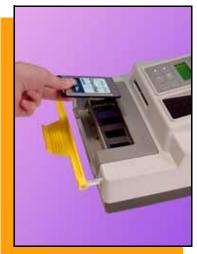
Periodically, updates to FlashPAK's internal operating system will be available. An update is loaded from a memory card or via an internet. Use TaskLink to copy the update onto the memory card (an "Update Card"), or to select the networked programmer.
