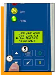
The Clean Alert number can be changed to display its cleaning message after a different number of insertions.
