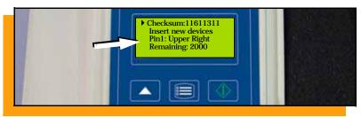
Most devices have a dimple located at pin 1. See manufacturers' specifications.
