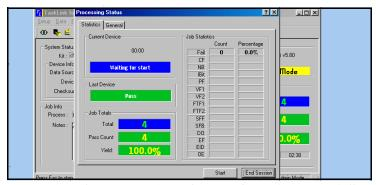
15. During the processing, the number of successfully programmed devices and total number of attempts is displayed. The **Last Device** box displays "Pass" on a green background or a message that describes failure on a red background.
