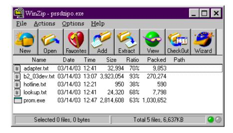
File b2\_03dev.txt is the Device List file used by TaskLink to update Device Database for OPTIMA programmers on PP100/PS-Series.
