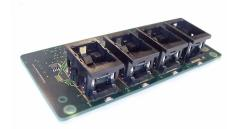
FlashPAK II supports both standard socket modules and High Performance (longer life) Socket modules
